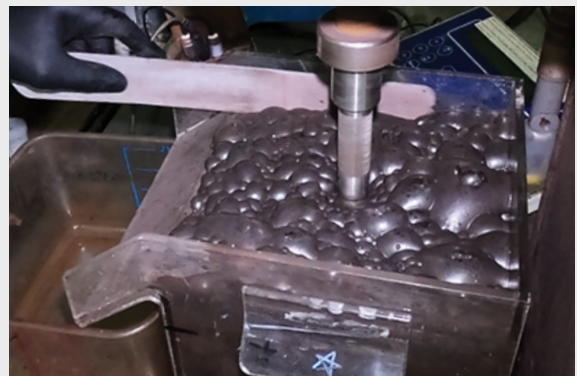
Saline Water Testwork | Bench scale flotation testwork at Bureau Veritas laboratories, Adelaide.
