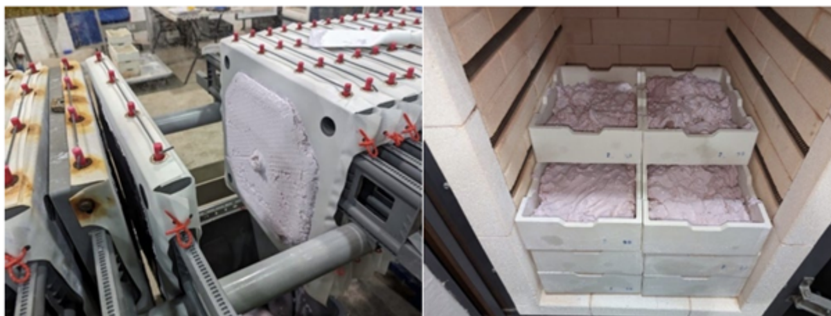
Figure 2: NdPr oxalate product produced post separation (left), and calcination feed (right).
