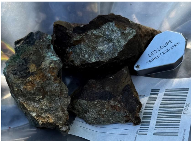
Figure 3 - Photograph of sample F005673, quartz-sulphide veining from Coyote which returned 17.4g/t Au, 1.47% Cu, 29.6g/t Ag.
