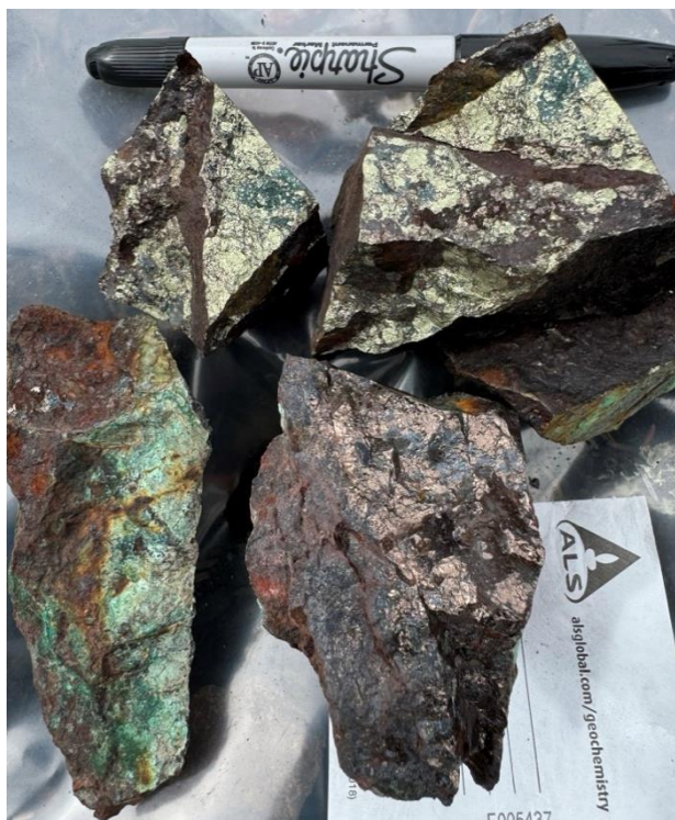
Figure 2 – Photograph of sample F005437 with massive bornite-chalcopyrite which returned 42.60% Cu, 2.28g/t Au, 159g/t Ag, 0.364% Co from the Glacier IOCG trend.
