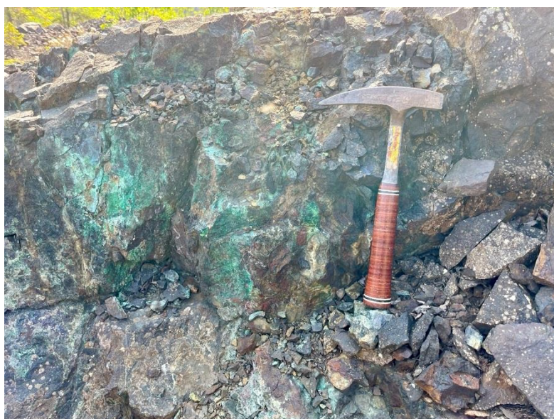
Figure 4 – Photograph of mineralised outcrop for sample F005604 which returned 716g/t Ag and 42.2% Cu at Payback.
