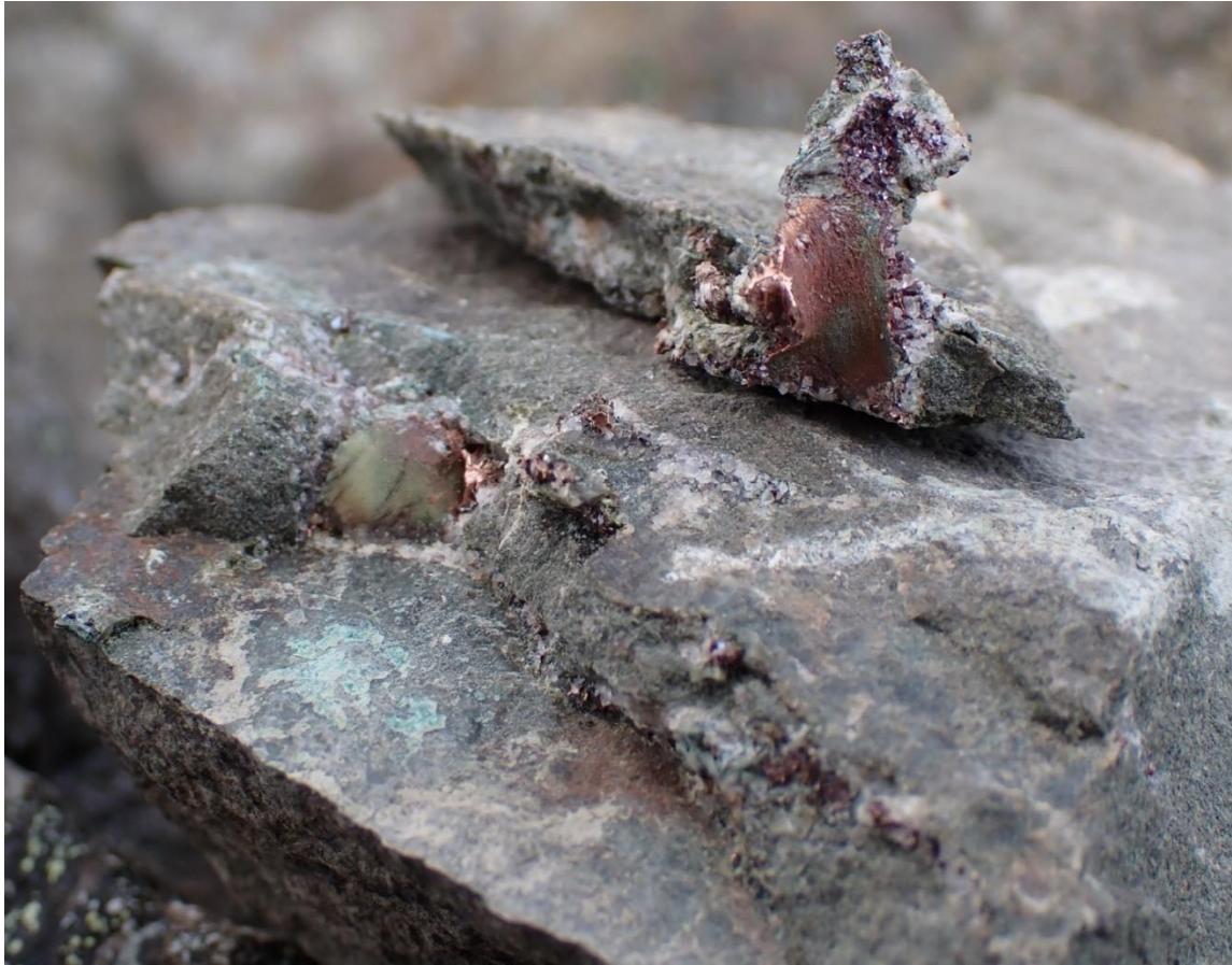
Figure 9 - Example of native copper mineralisation from the southern extent of the HALO vein system. Field of view 10 cm. (Sample F005999).
