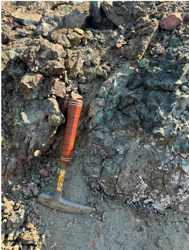
Figure 6 – Outcrop photograph for sample F005408 illustrating a brick red K-feldspar-skarn breccia with abundant copper secondary minerals after chalcopyrite-bornite-chalcocite sulphides. Sample returned 233g/t Ag, 9.82% Cu, 1.67% Pb, 2.35% Zn .
