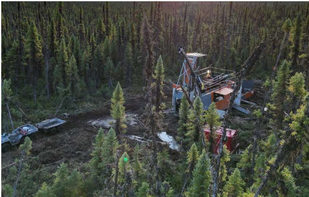
Figure 4: Diamond drill rig operational on hole POM-23-013 at the Pomme project, August 2023.
