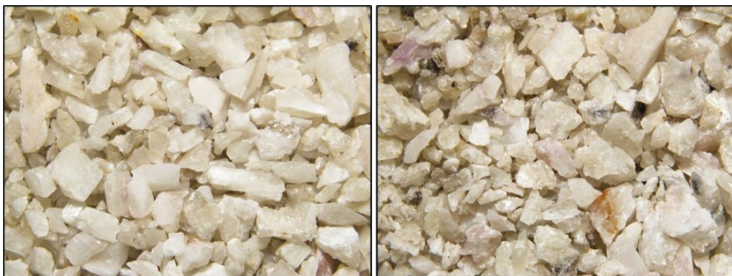
Figure 8: HLS concentrate fractions grading ~6.0% Li 2 O (left) and ~5.5% Li 2 O (right)
