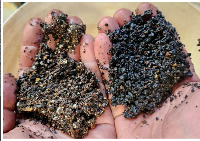
Figure 7: DMS separated material from KR1 showing beneficiated manganese ore on the right side and waste to the left.
