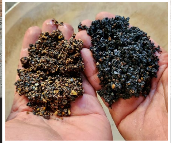
Figure 8: DMS separated material from KR2 showing beneficiated manganese ore on the right side and waste to the left.
