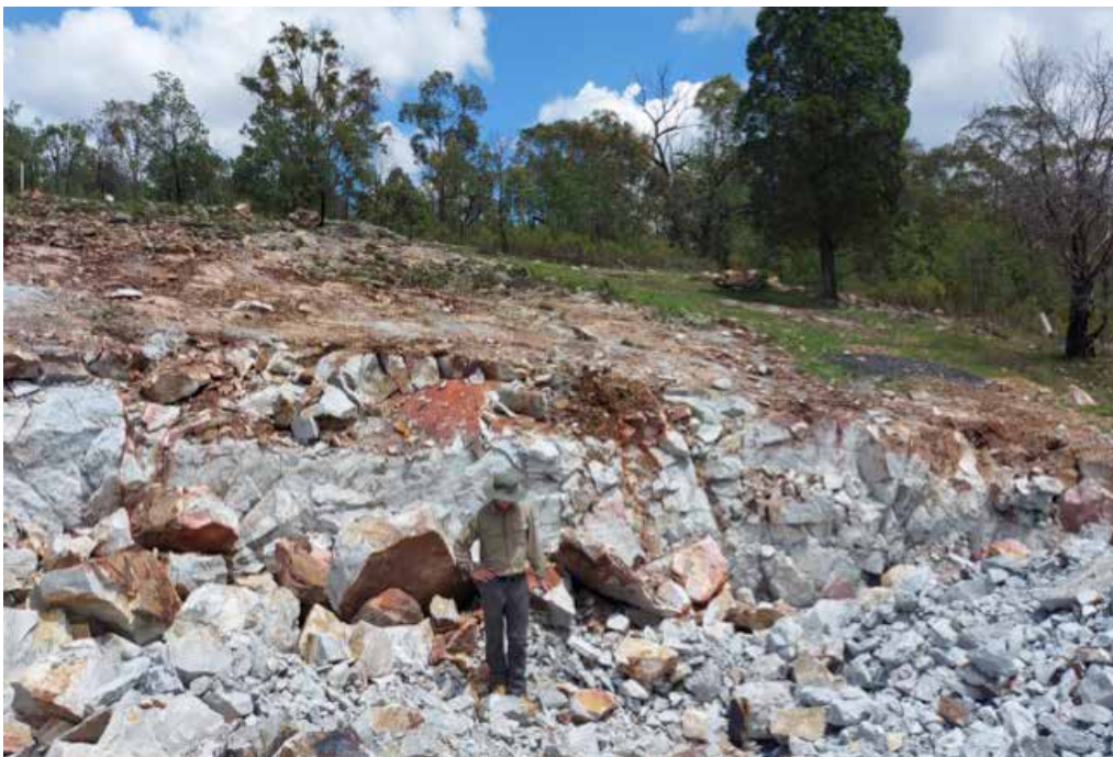
Figure 7: bulk sample blast site showing mineralised fractures.
