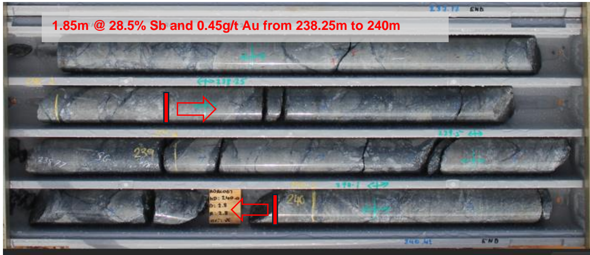
Figure 14: Photo of RDRC067 core tray from 237.17 – 240.41m, representing part of the high-grade Sb interval; extremely altered and brecciated ultramafic. Sb is occurring primarily (but not exclusively) as breccia.
