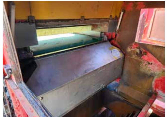
Inside TOMRA Ore Sorter #2 showing the valve bank (left) and the end of the conveyor belt where the material gets ejected (right).
