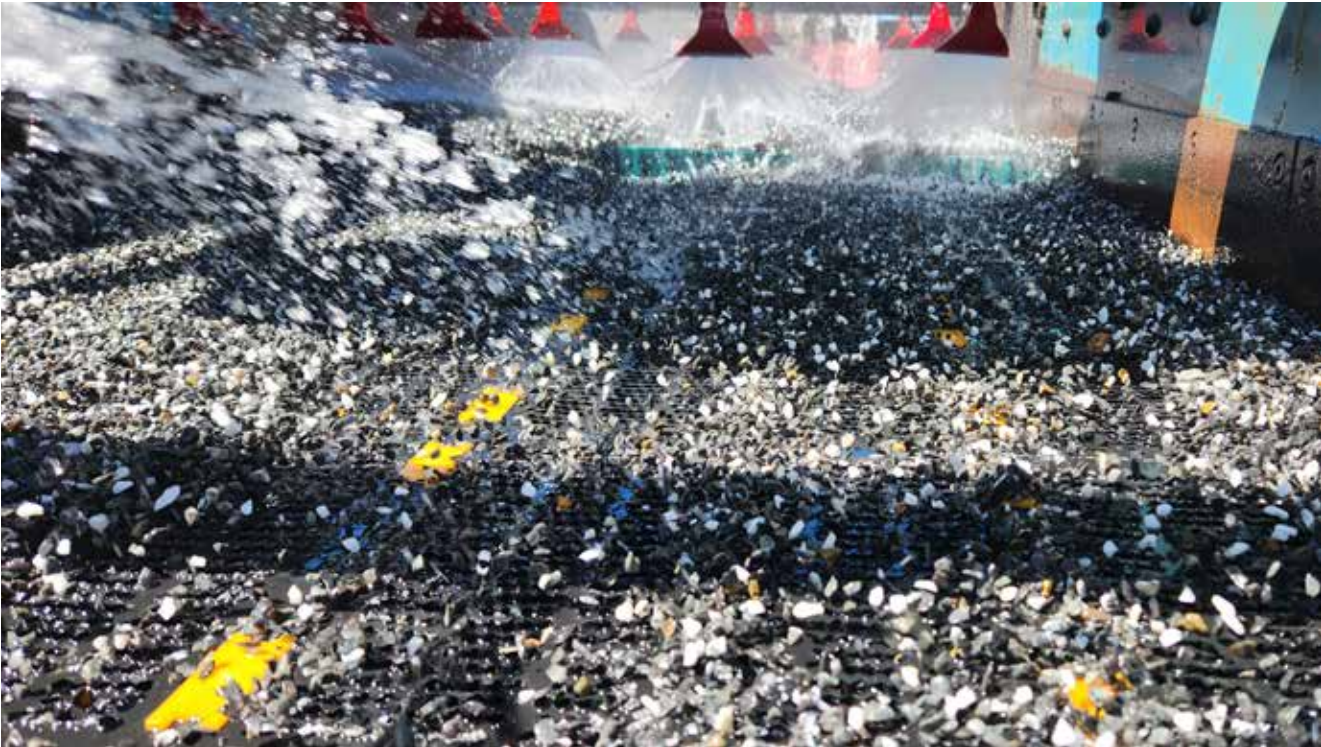
Fine ore being screened in a vibrating screen with new self-cleaning panels, ahead of the Mineral Jig at the Gravity Plant.
