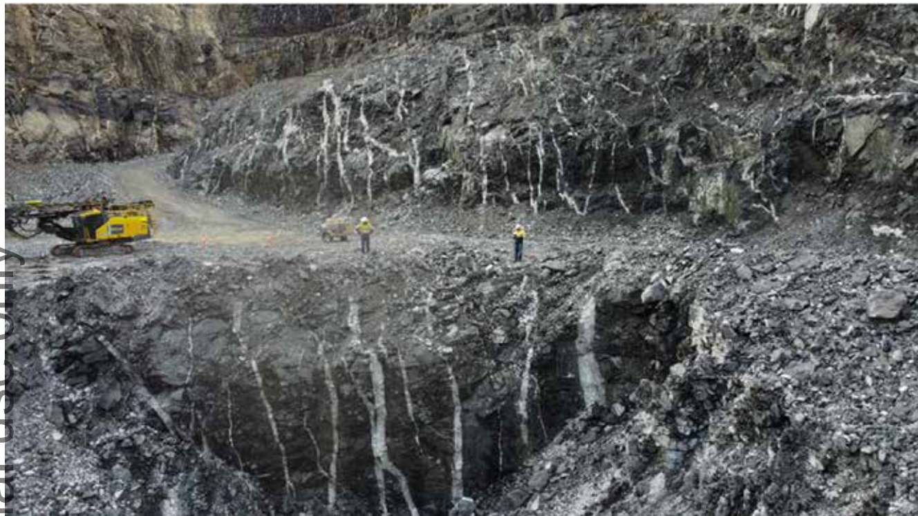
Johnson veins showing up in the pit – looking at blast # 305-002 wall. Individual vein's look high by visual inspection with the entire face being 0.28% WO 3 in this region.
