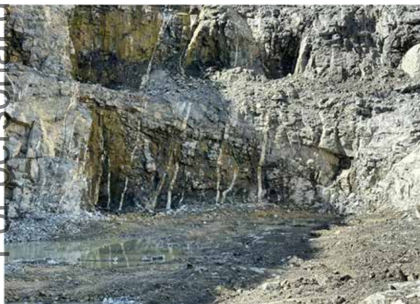
Level 295m RL confirms the thickening of the veins as seen on the cliff face looking into the Johnson Vein system.
