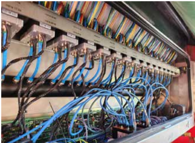
Inside TOMRA Ore Sorter #2 showing the valve bank (left) and the end of the conveyor belt where the material gets ejected (right).
