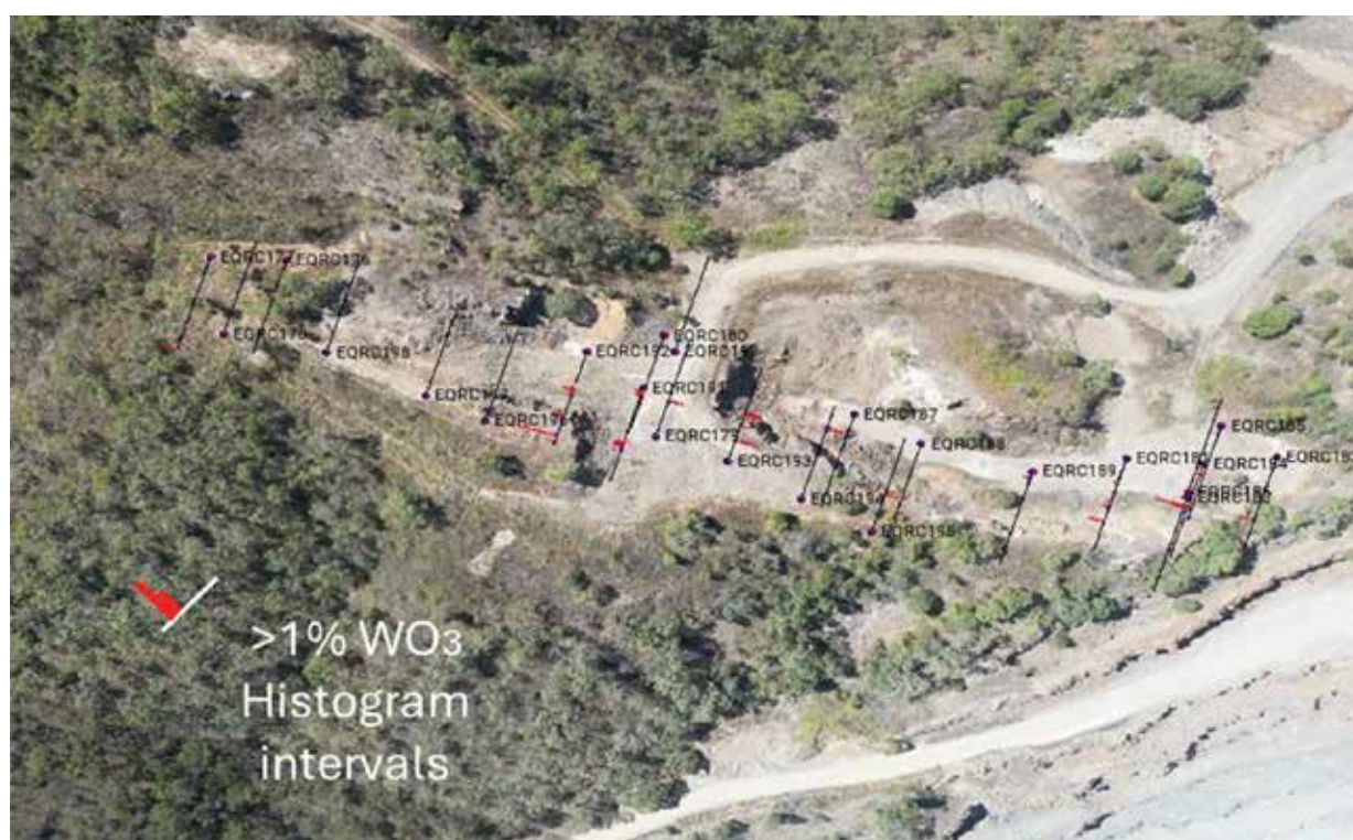
Ruby Vein section & plan showing thin veins at high level in the system. Shallow 50-meter holes hit 12 meters of grades up to 1.2% \text{WO}_3 .
