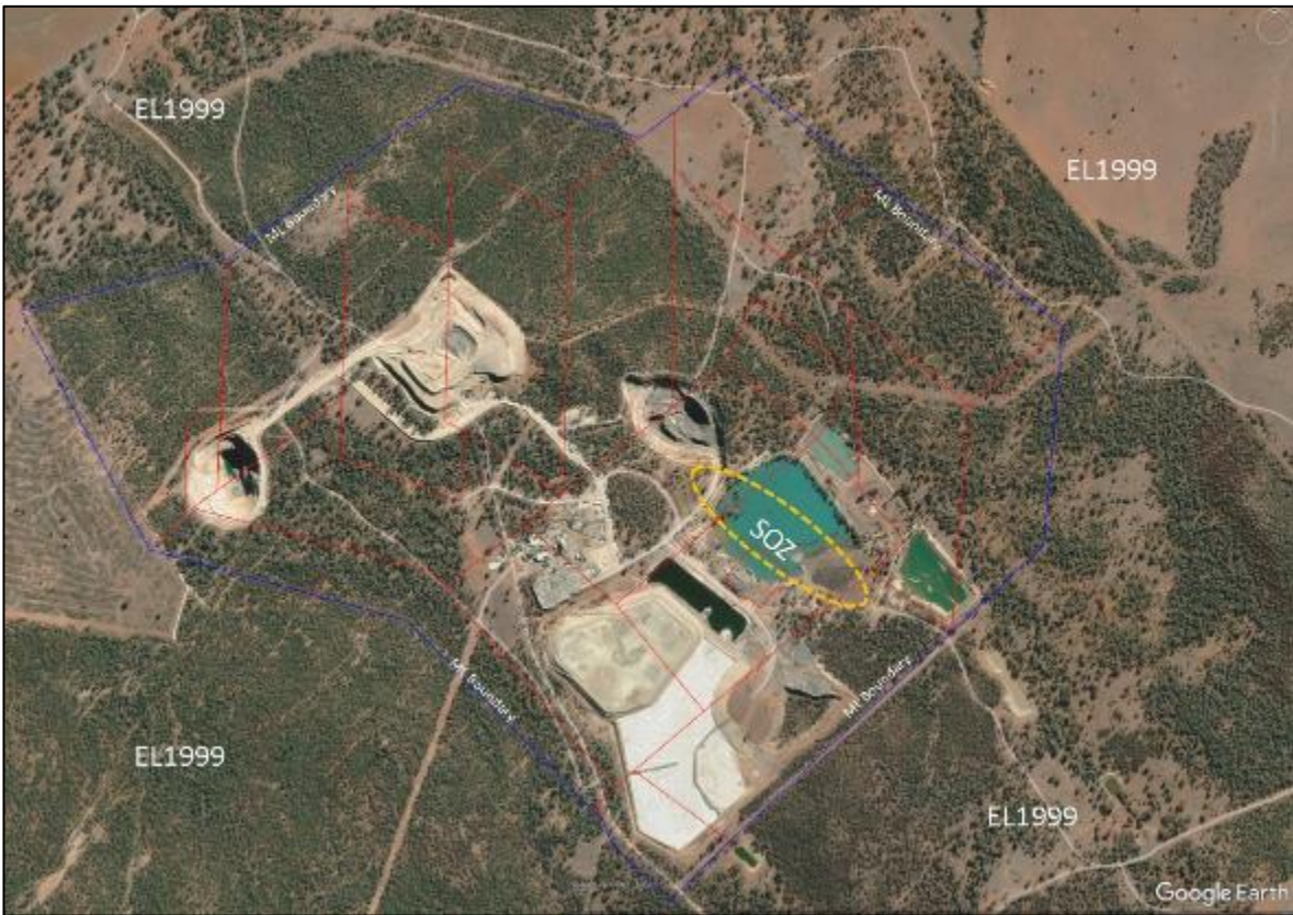
Figure 8 Mineral Mill Mine - Mining Lease areas with surface projection of the location of Southern Ore Zone deposit
