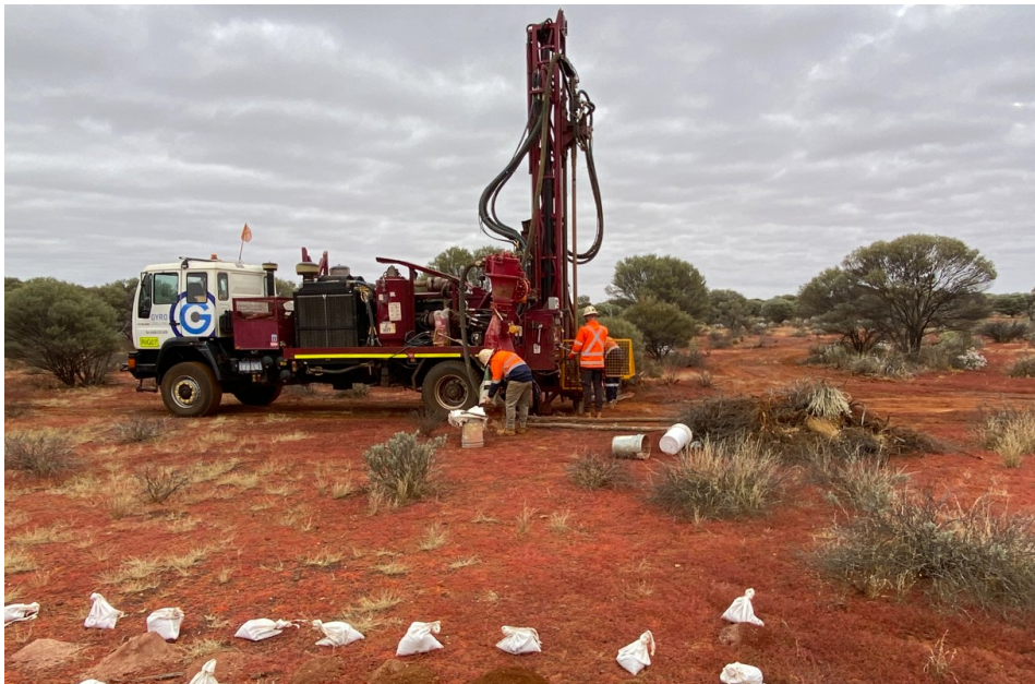
Figure 4: Aircore drill rig in operation at E38/3997
