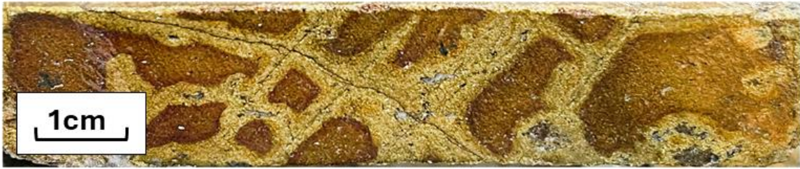
Figure 3 – Photo of diamond core completed by Australian Oil & Gas Minerals Pty Ltd (1970's). Sample interval of 4.6 metres at 18.54 % Cu from 57.9 metres in TDH01 containing massive chalcopyrite (copper sulphide). Core diameter is BQ (36.4mm) with quarter core retained as a representative sample. Chalcopyrite is tarnished brown by length of time in core tray.
