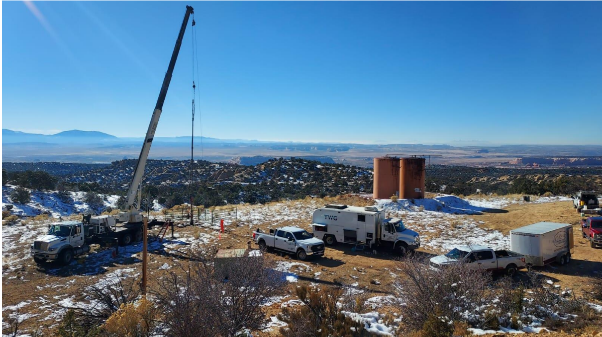
Figure 2. Wireline unit conducting brine sampling operations
