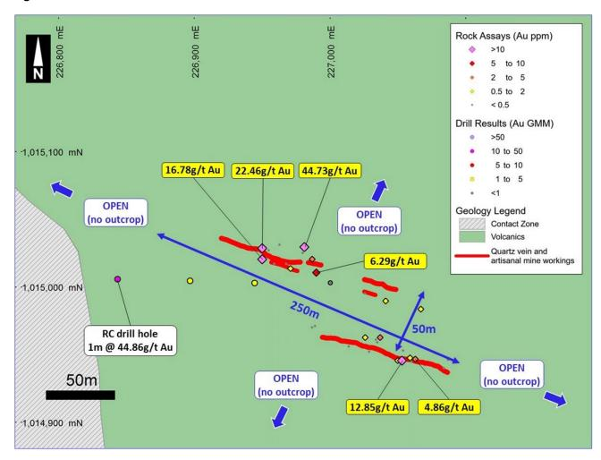
Figure 8: Double Zone - High-grade rock chips results along new east-west structures in artisanal workings with gold-bearing quartz veins
