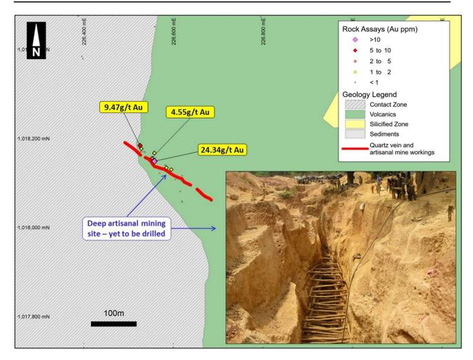
Figure 9: Rock chip samples from spoil piles returned very high-grade values even though they were collected from miners' rejects
