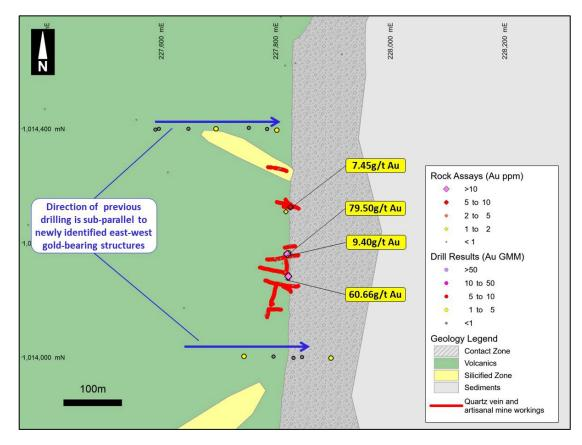
Figure 6: Ladder Zone - High-grade rock chips results along new east-west structures in artisanal workings with gold-bearing quartz veins – note that the majority of veins are east-west and previous drilling would not have intersected the east-west structures
