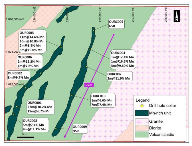
Figure 19: Ouangolodougou Permit with reconnaissance drill hole location and results - There is only one drill hole at each location and average drill hole spacing is over 1km apart
