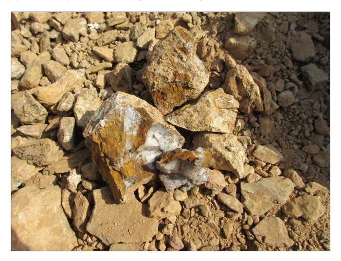
Figure 7: Rock chip sample of quartz veins from spoil pile which returned 79.50g/t Au
