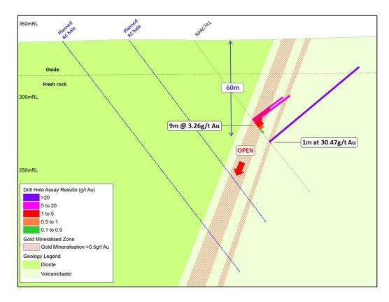
Figure 17: Cross section from previous scout drilling at artisanal mining site which returned rock chip samples up to 170g/t Au from spoil piles
