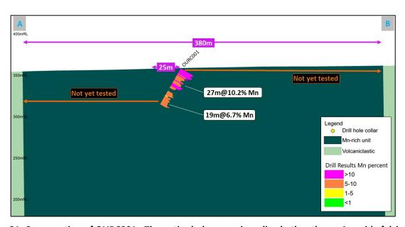
Figure 21: Cross section of OURC001 - The entire hole was mineralised other than a 4m wide felsic dyke - Only 25m of the interpreted 380m width was drill tested
