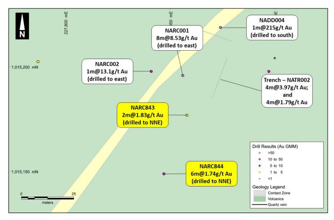
Figure 13: Discovery Zone – Select new (yellow) and previous (white) drill intercepts-Note that gold is intersected in multiple drilling directions suggesting multiple events of gold mineralisation
