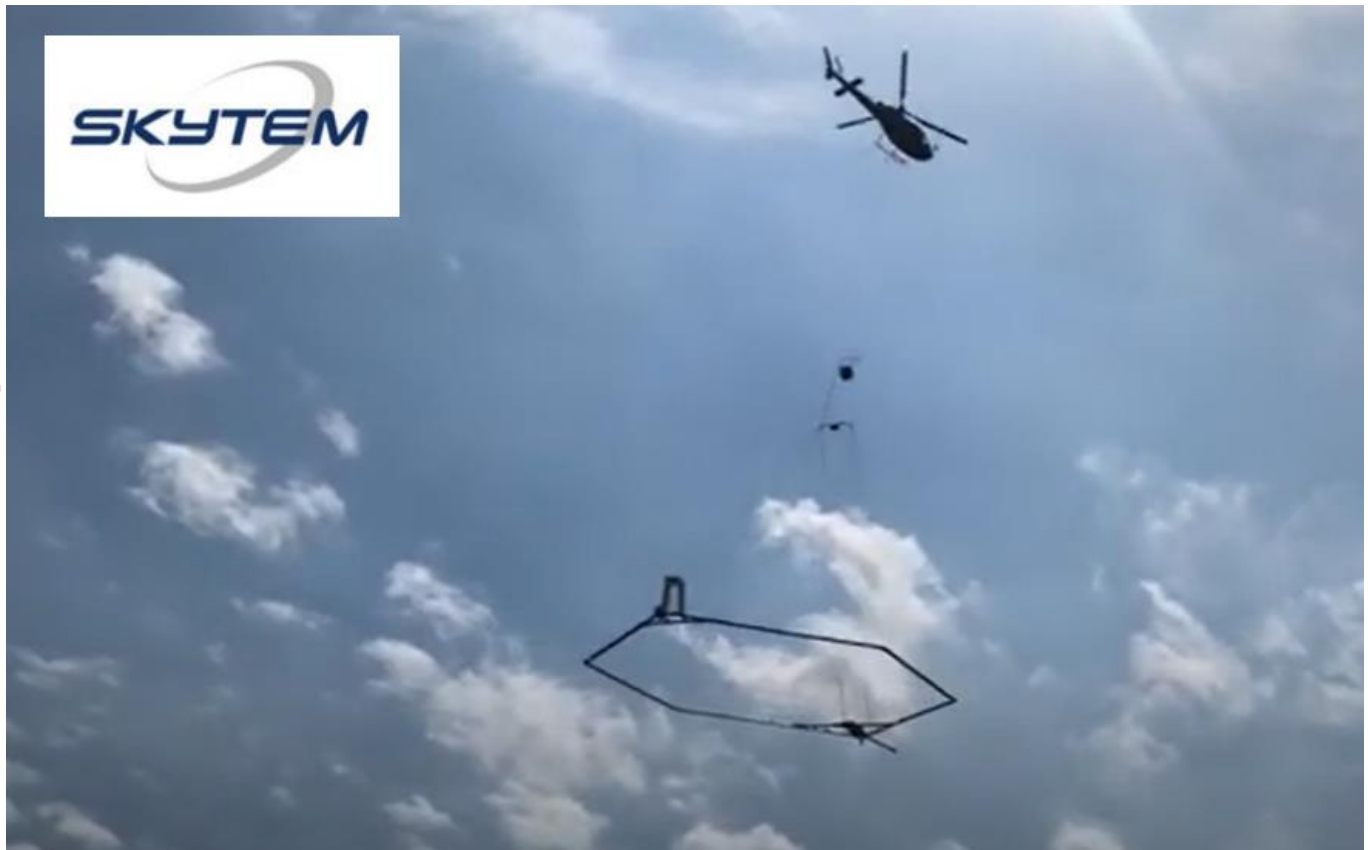
Figure 9 - SkyTEM's low-frequency time domain EM and magnetic system. proposed to complete a detailed heli-borne EM survey over the Maniopota prospect (Ruddygore Project) and funded by a Queensland State Government CEI grant.
