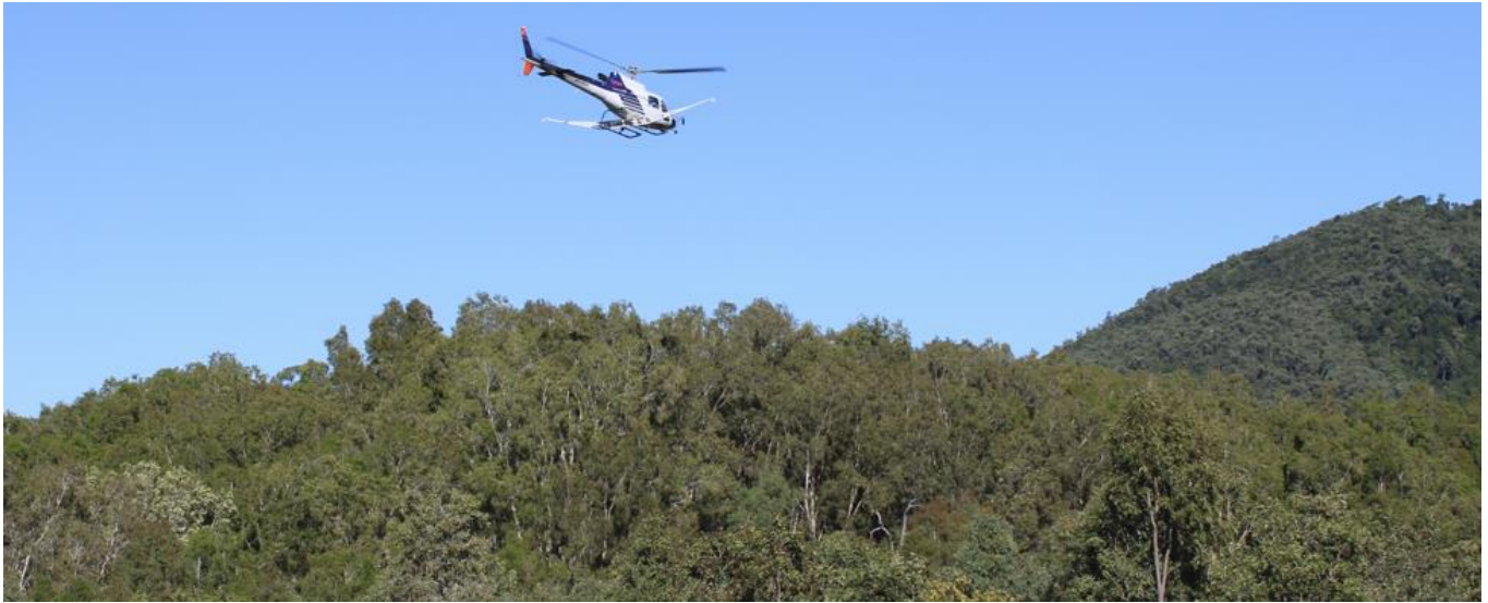
Figure 5 - NRG's Xplorer™ heli-borne magnetic survey being flown over the Dittmer project area and funded by a Queensland State Government CEI grant.
