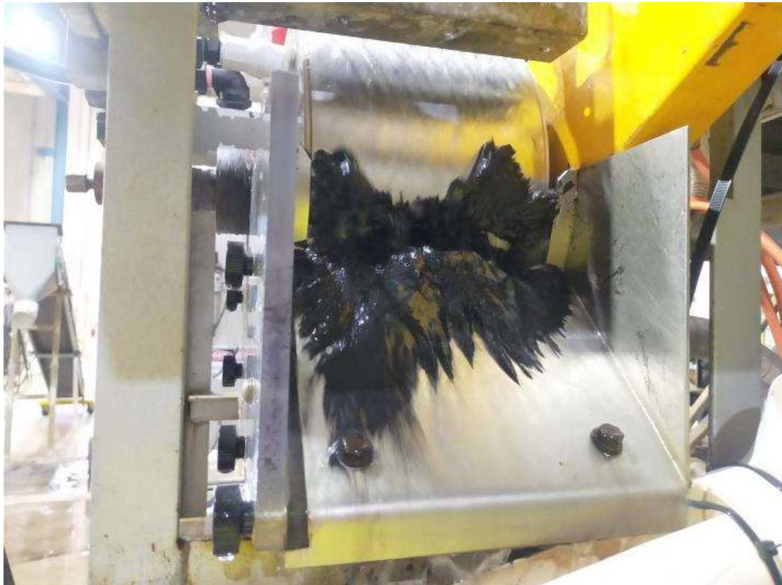
Plate 3 – Magnetite concentrate from large scale pilot plant operation
