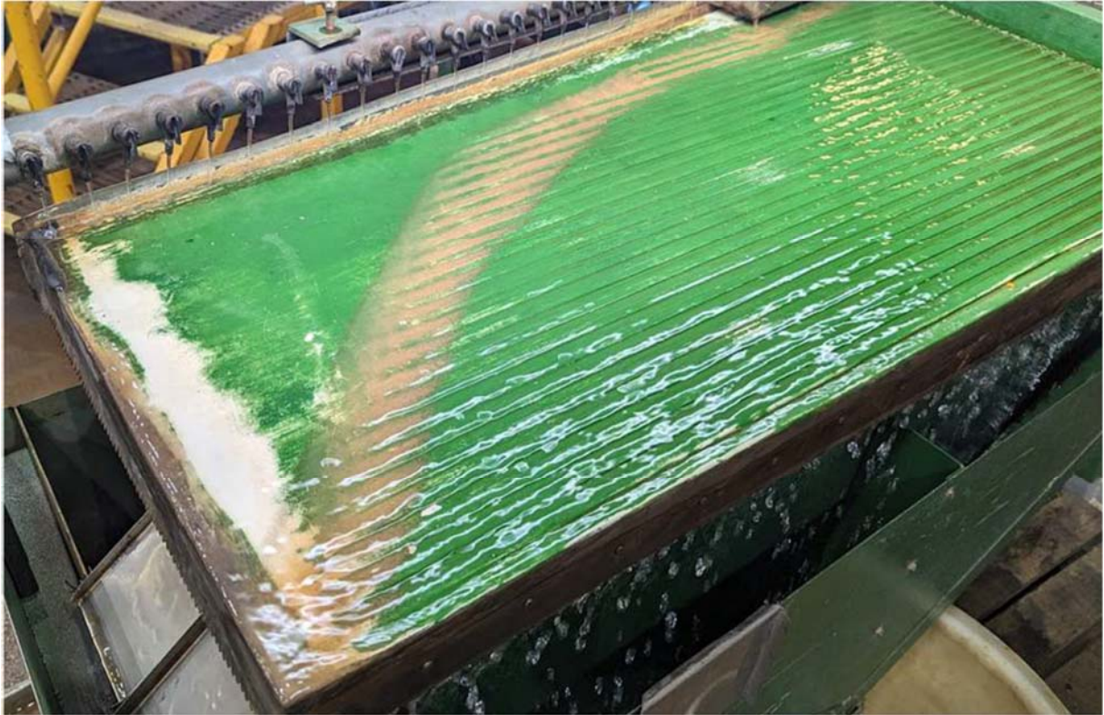
Figure 7: Wet shaker table separation simulating a plant cleaner stage.
