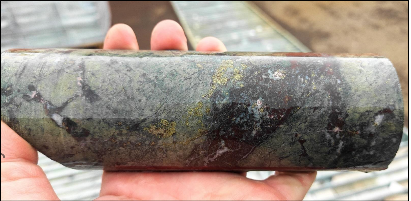
Figure 7. Photo of gold-copper-zinc mineralisation from 471.6m down-hole depth – 1.3g/t Au, 0.6% Cu, 2.1% Zn and 6.8g/t Ag.
