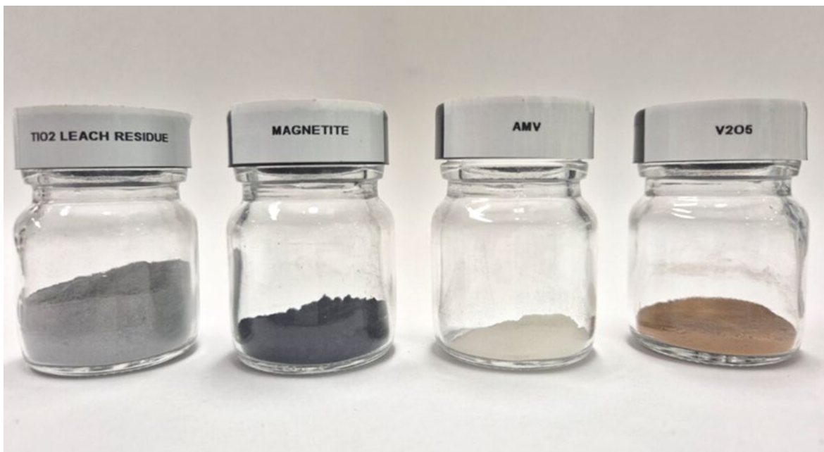
Figure 1: Samples – titanium dioxide (leach trials), magnetite (iron recovery trials), “AMV” (ammonium metavanadate is a pre-cursor to the V 2 O 5 (preparation) and vanadium pentoxide (Source: CSIRO)
