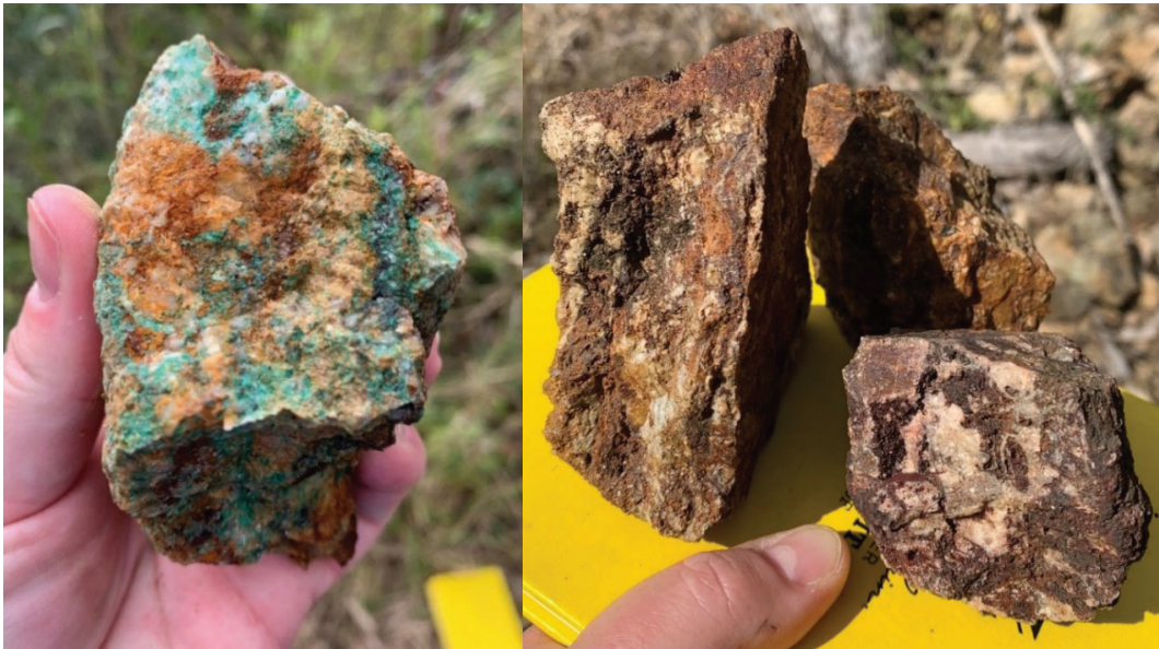
Figure 3. Sample MRRK071, 3.49g/t Au, 2.8% Cu & 195g/t Ag (left). Sample MRRK072, 6.06g/t Au, 585g/t Ag, 1.5% Cu, and 3.58% Sb (right).
