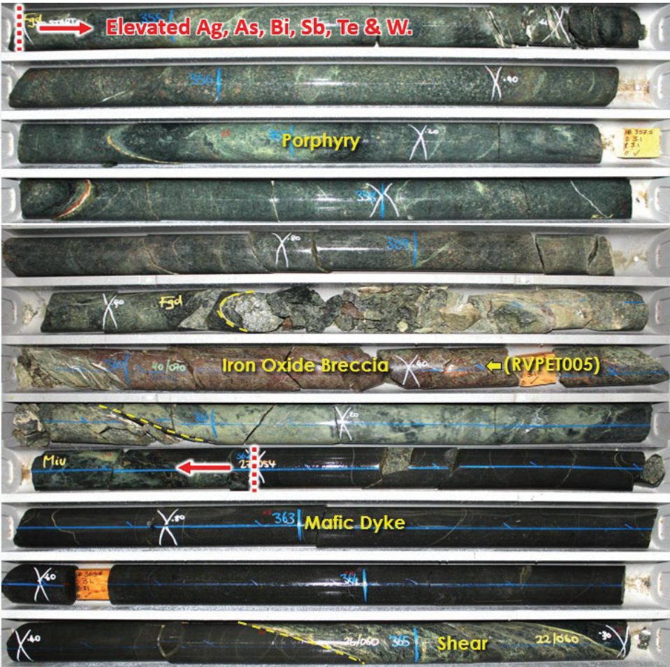
Figure 16. 7.2m zone of interest within diamond core (RVCD0006), 354.8 – 362m, containing a porphyry, iron-oxide breccia, and a mafic dyke. Multi-element assay results returned 7.2m @ 0.32g/t Ag from 354.8m 16 .
