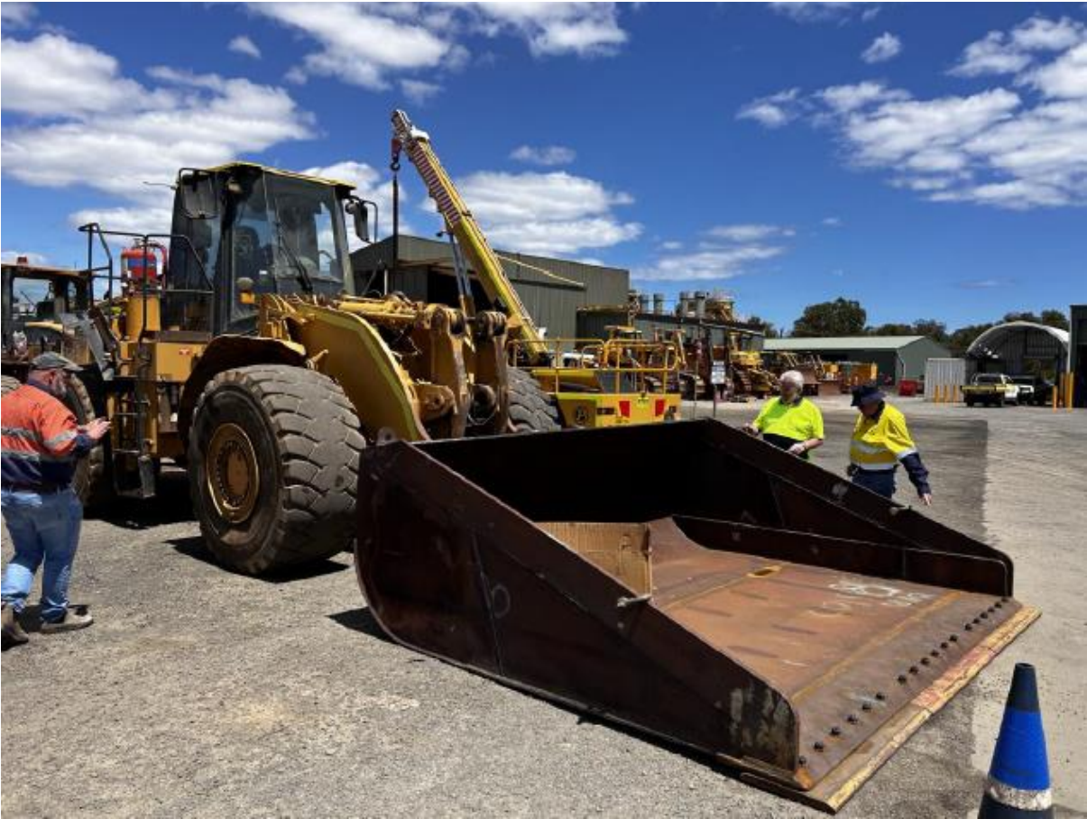
Modified front-end loader bucket for VDT mining method
