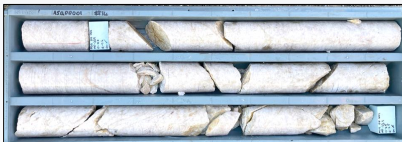
Diamond Drill Core – Quartz Hill MGSI Deposit
