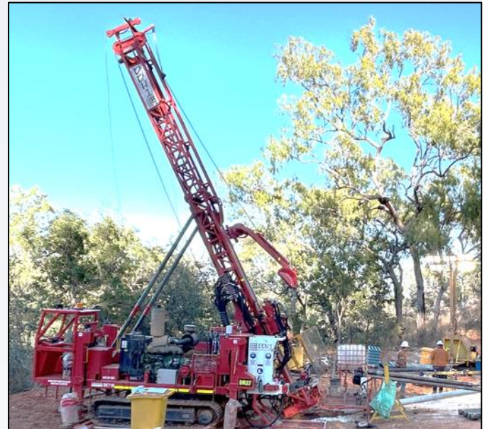
Diamond Drilling of Hole ASQDD001 in July 2024
