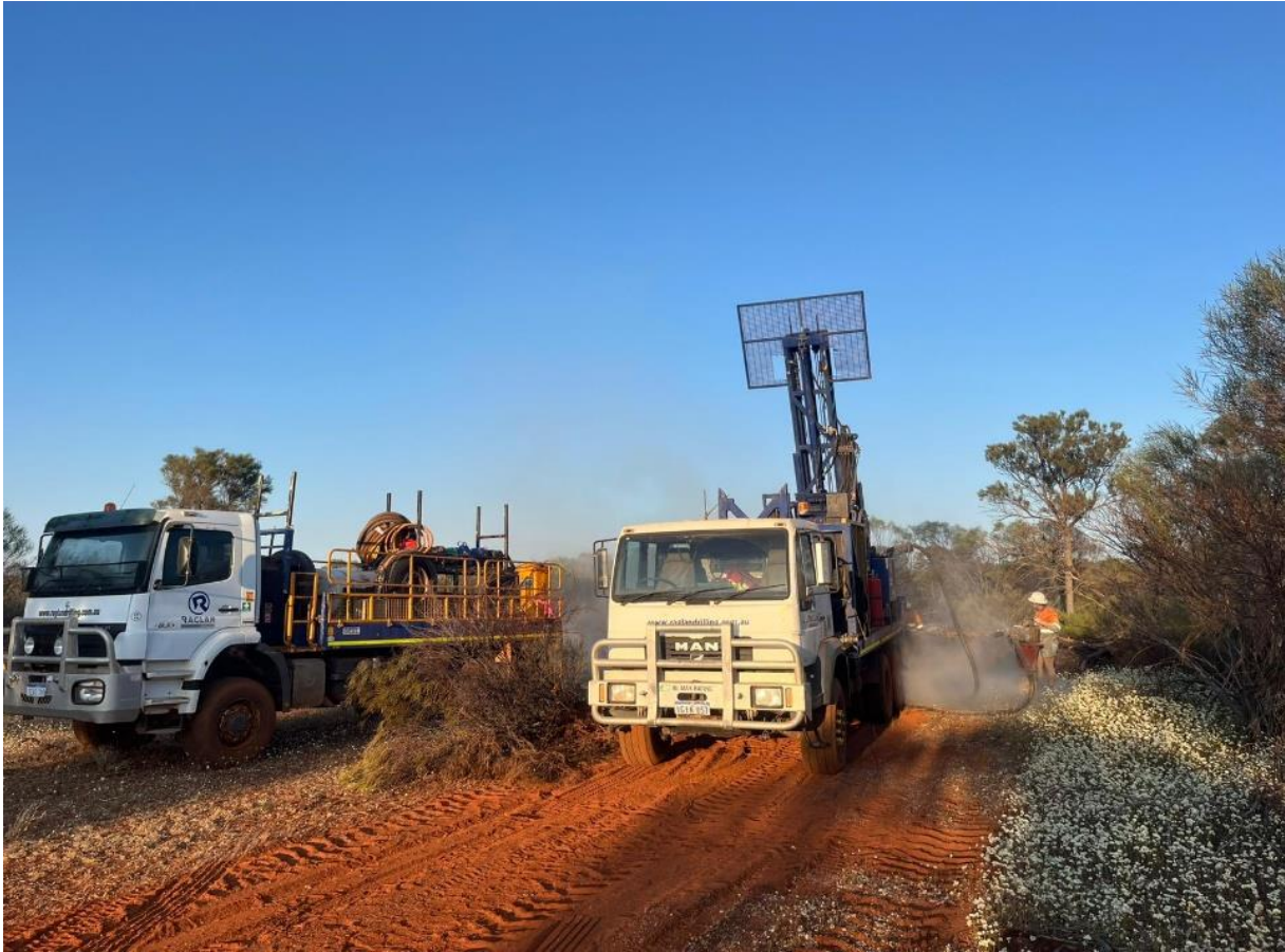
Picture 2: Ragland AC rig and support vehicles on site at Wildflower.
