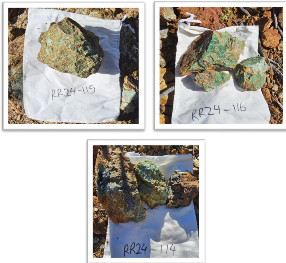
Figure 6. Rock chips taken for copper mineralisation at the Reward Cu-Au-Ag Prospect. RR24-116 assayed 19.5% Cu, 3.2g/t Au and 2,090.0g/t Ag, RR24-115 assayed 19.6% Cu, 12.2g/t Au and 781.0g/t Ag and sample RR24-114 assayed 13.8% Cu and 19.4g/t Ag.
