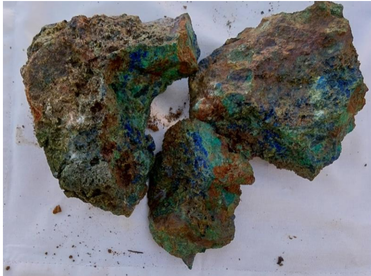
Figure 1. Sample PER056, recently collected near shallow workings at the central-southern portion of the Black Ridge trend during reconnaissance mapping. The sample contains secondary copper carbonates (blue and green) in an altered andesite host, with assays for the sample returning 7.5% Cu & 23g/t Ag . See Table 1 for full sampling details.
