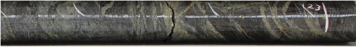
Figure 9: Photograph of core from BHRC030, 123m showing quartz-pyrite veins \pm chalcopyrite-molybdenum
