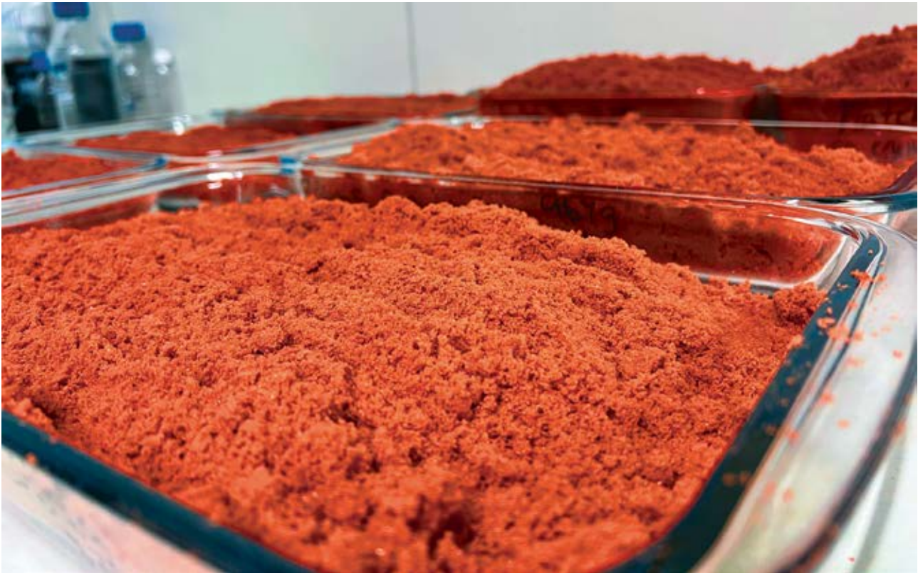
Figure 18 – Cobalt Sulphate crystals produced from third-party feedstocks
