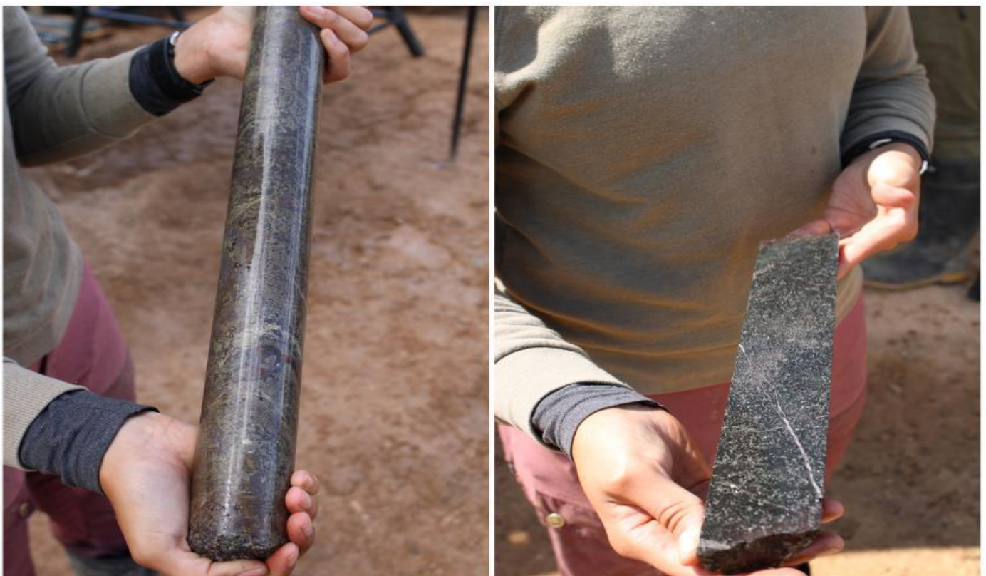
Figure 5: W56 prospect -WL23-367: 21.9m @ 1.02% Ni from 206.65m including 1.35m @ 5.02% Ni from 227.2m and 4.4m @ 1.55% Ni from 247.1m. Massive Sulphides at 227.2m and net texture sulphides at 248.5m, refer ASX on 11 July 2023.
