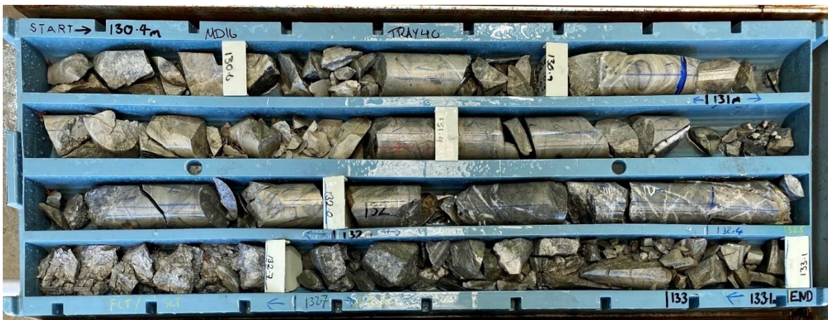
Figure 3. MD16 (127.65 m – 133.1 m). Leven Star Reef intersection in fresh sulphide material (14.0 m @ 6.15 g/t Au from 120 m, including 7.60 m @ 6.66 g/t Au from 121.9 m and 3.0 m @ 11.06 g/t Au from 131 m) 5 . Peak gold assay is associated with a discrete sulphide rich fault breccia and increased quartz stock-work veining. Intercepts are expressed as down-hole intersections and should not be presumed to represent true widths, which vary from hole to hole and between reefs (refer JORC Table 1).
