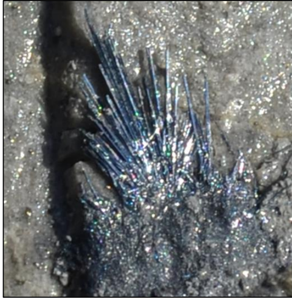
Figure 2: Stibnite (antimony sulphide) needles in fracture in core from BPD08. Antimony containing minerals at Bulla Park are tetrahedrite and stibnite.
