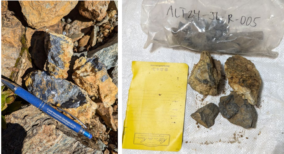
Figure 4: Massive stibnite (90-100%) in subcrop shear zone associated with quartz. Shear is steeply dipping and striking east-west, with cm-scale stibnite pieces visible.
