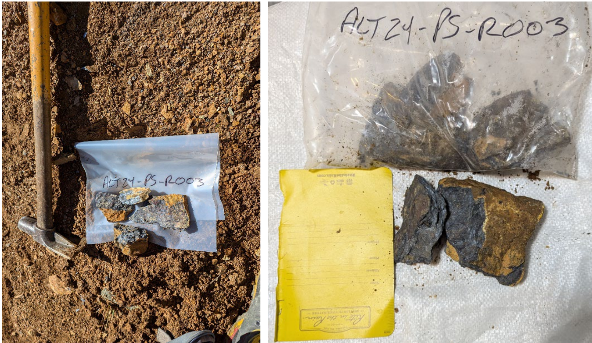
Figure 2: Subcrop sample of massive to platy silver-grey stibnite (90%) with orange-brown staining. Limited quartz (<3%) is present, with fine to coarse graining and minor quartz vugs. This sample is representative of strong mineralisation along the shear zone.
