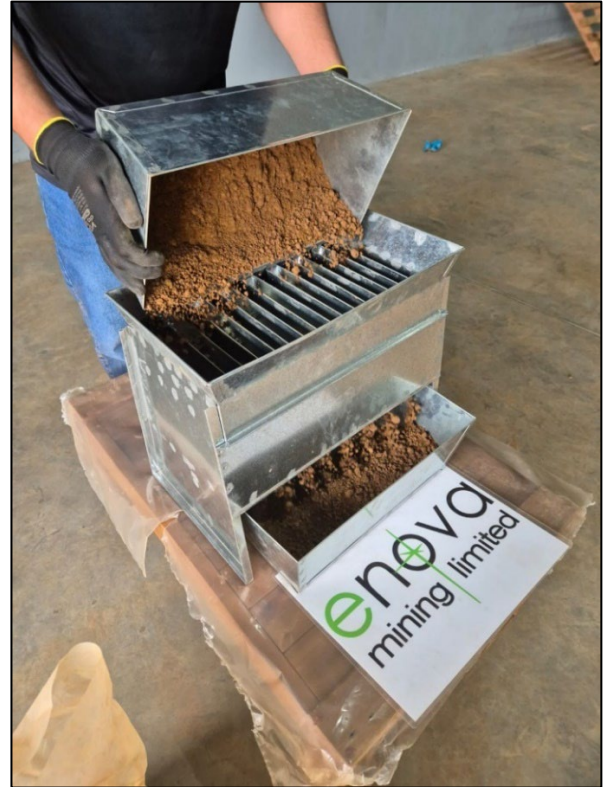
Figure 7: Enova professional geologist sub-sampling by using riffle splitter
