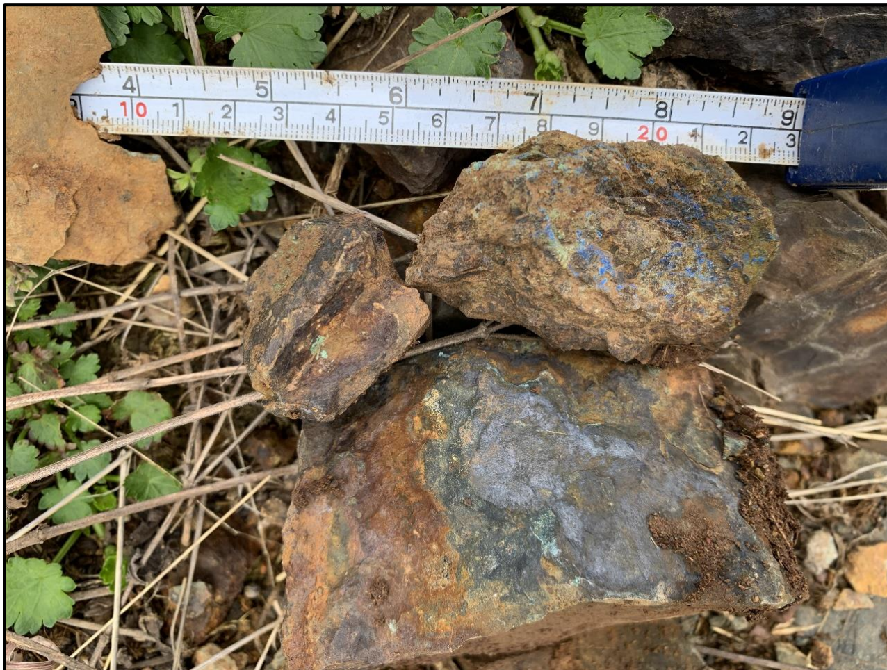
Image 2: Milfor prospect, altered Sofala Volcanics (basalt) with copper mineralisation (chalcopyrite, malachite)
