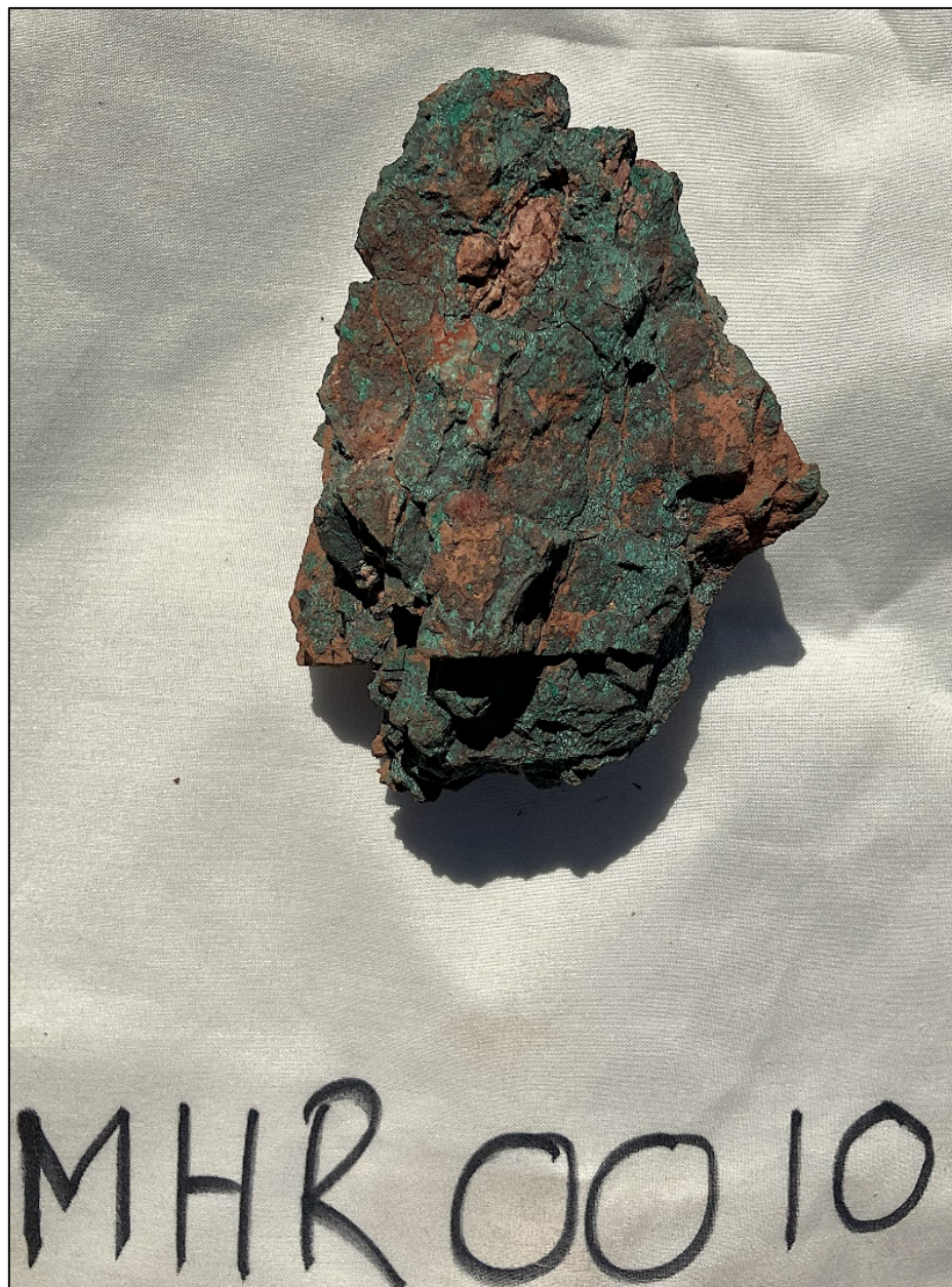
Photo 1: Sample MHR0010 which returned a grade of 45.5% Cu. Sample is ~7cm across
