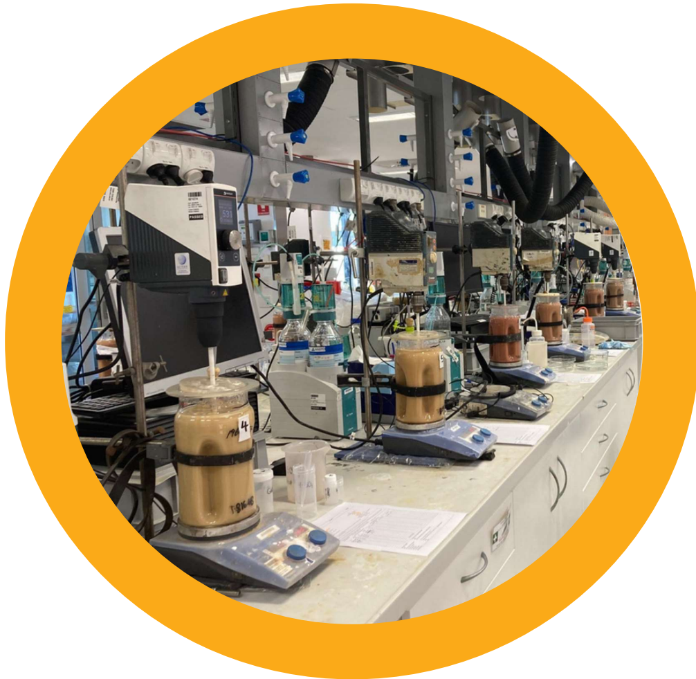
Figure 2: Diagnostic leach tests being conducted in the ANSTO Minerals Leach Laboratory, Sydney, NSW.
