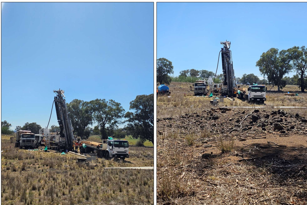
Figure 5: Drill rig at drill hole GYVRC001 (Cyclops) – photos are looking generally northeast with drill hole inclined at 60 degrees to 220 degrees (True North). Note old workings on lode material on right hand side.
