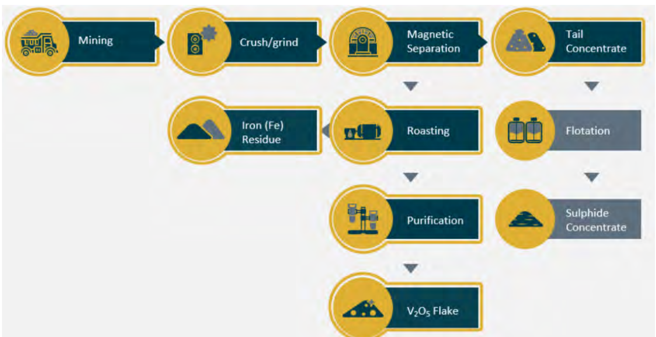
Figure 6: Schematic diagram showing industry standard flowsheet stages used to process Canegrass mineralisation with the stages completed to date (dark blue) and the stages yet to be completed (grey).
