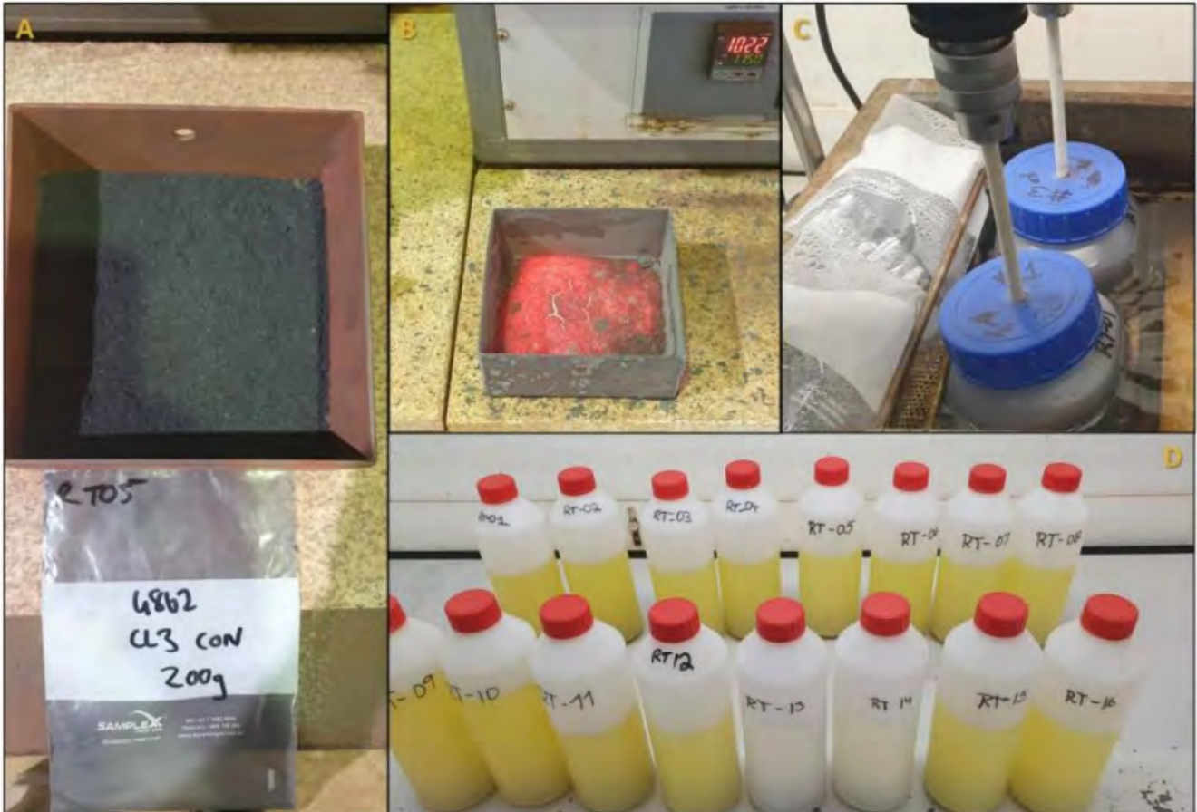
Figure 5: Photos showing A) Magnetic concentrate prior to roasting, B) Sample removed from oven after roasting, C) Water leaching from roasted sample & D) Filtered liquor containing leached Vanadium.
