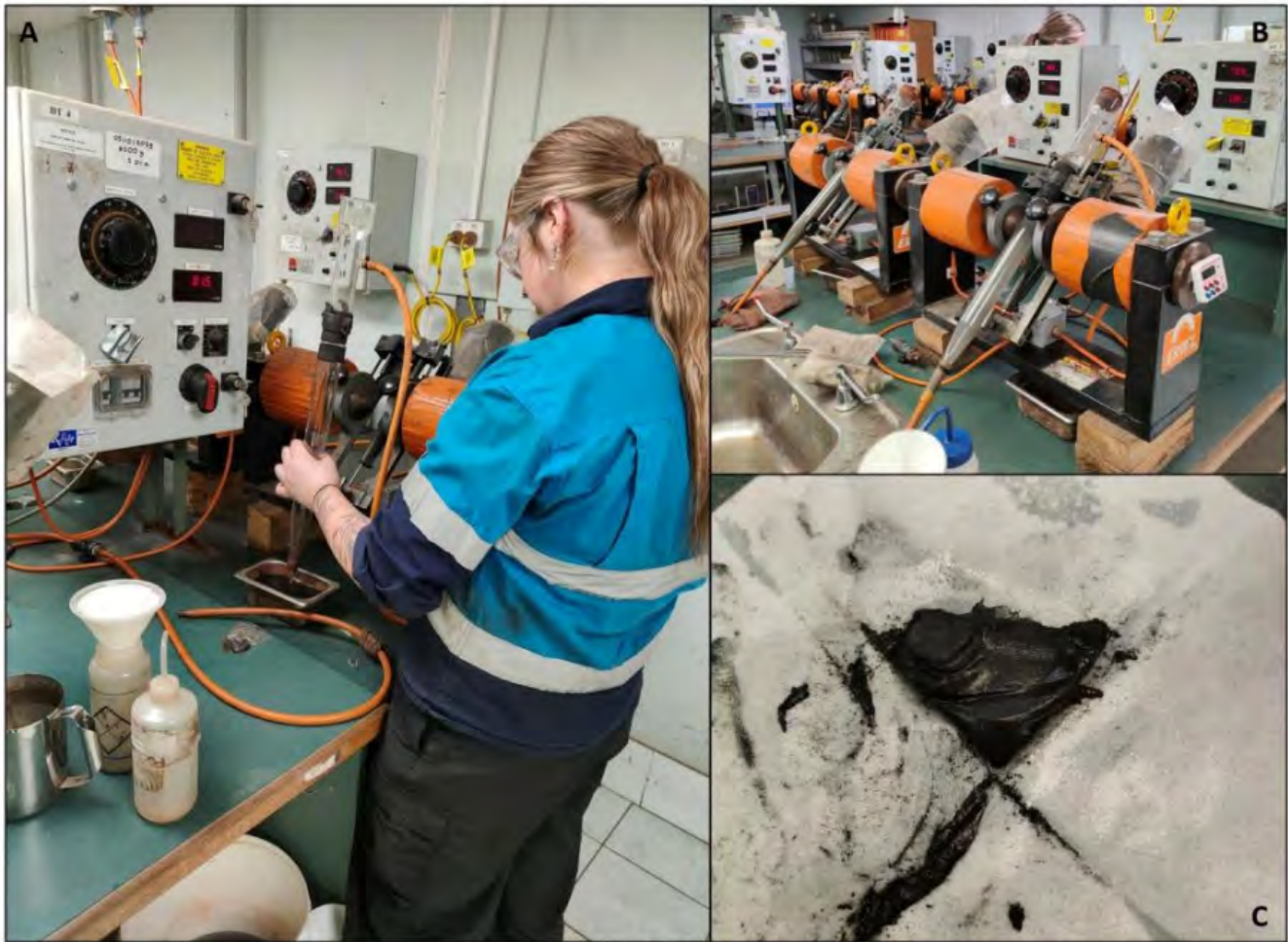
Figure 4: Photos showing A) Samples being prepared for filtration after DTR testwork completed, B) Eirez Davis Tube tester setup for sighter DTR testing and C) Magnetic concentrate produced after filtration.
