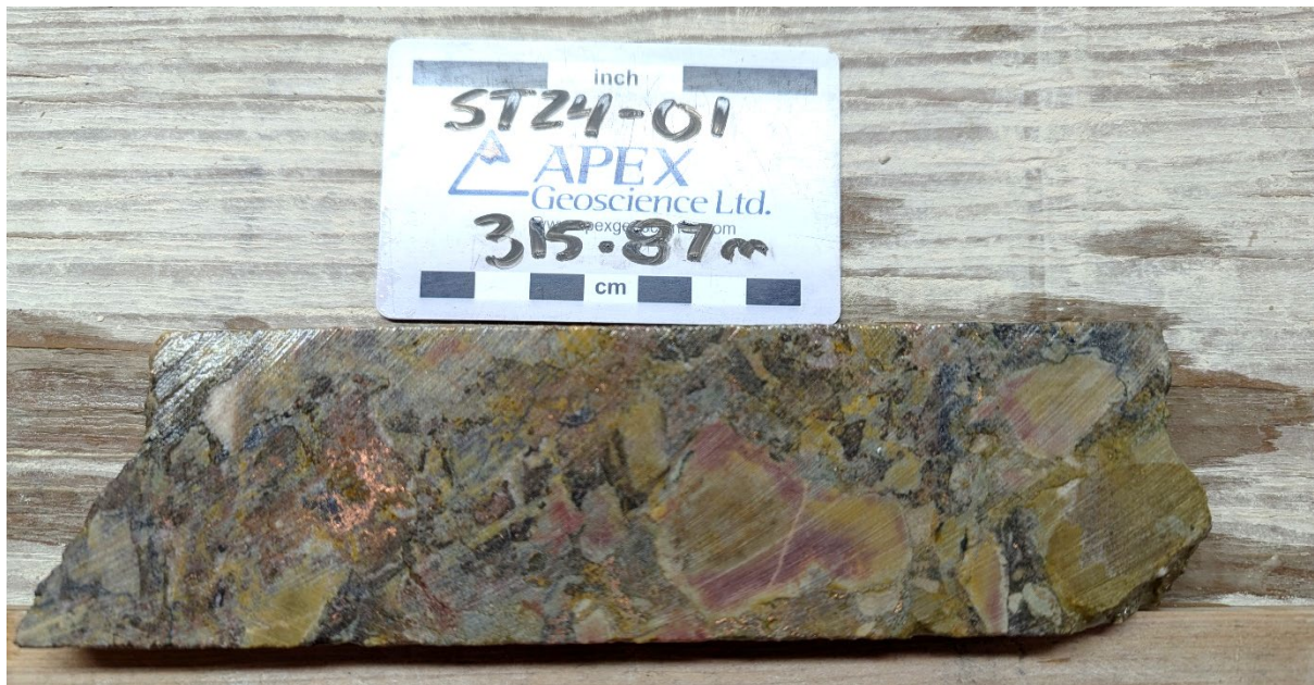
Figure 1: Chalcocite (dark grey) breccia and native copper (metallic) blebs within fractured dolomite in drill hole ST24-01 from approximately 315.87m downhole. This interval assayed at 3.7% Cu.
