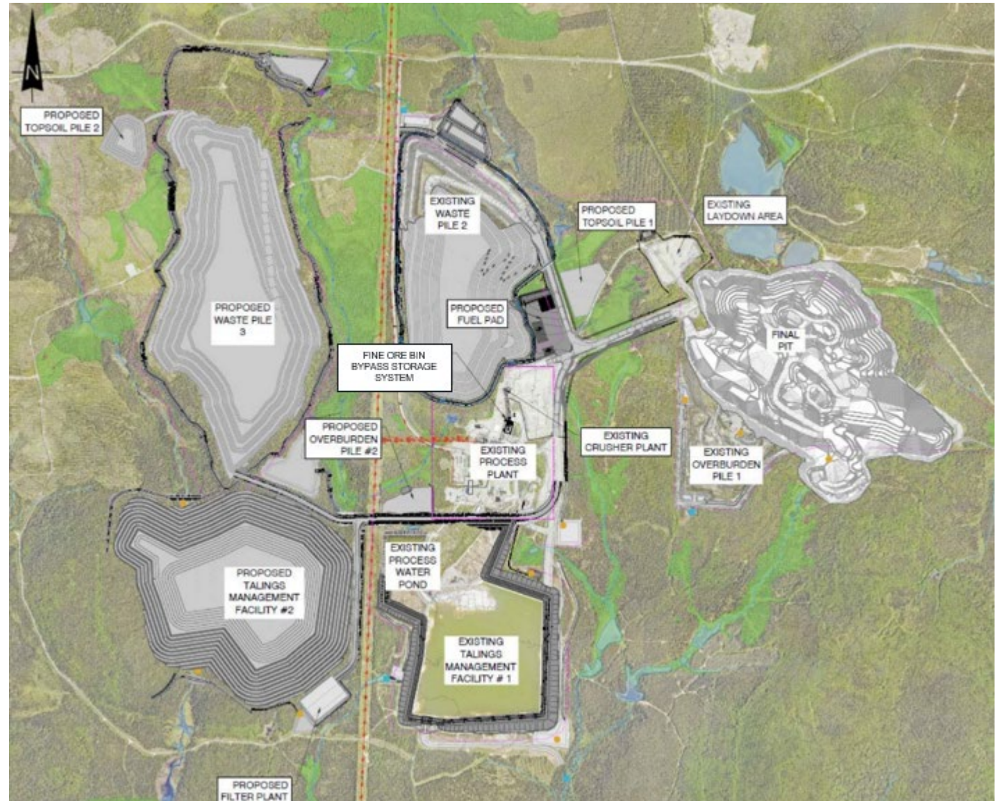
Figure 1 : NAL Site Layout Schematic (DFS 2023)
