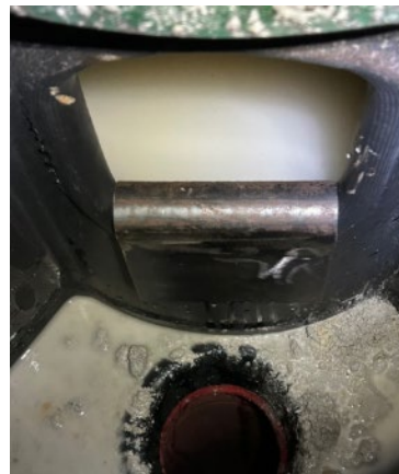
Picture 3: New stack sizer screen feed inserts
