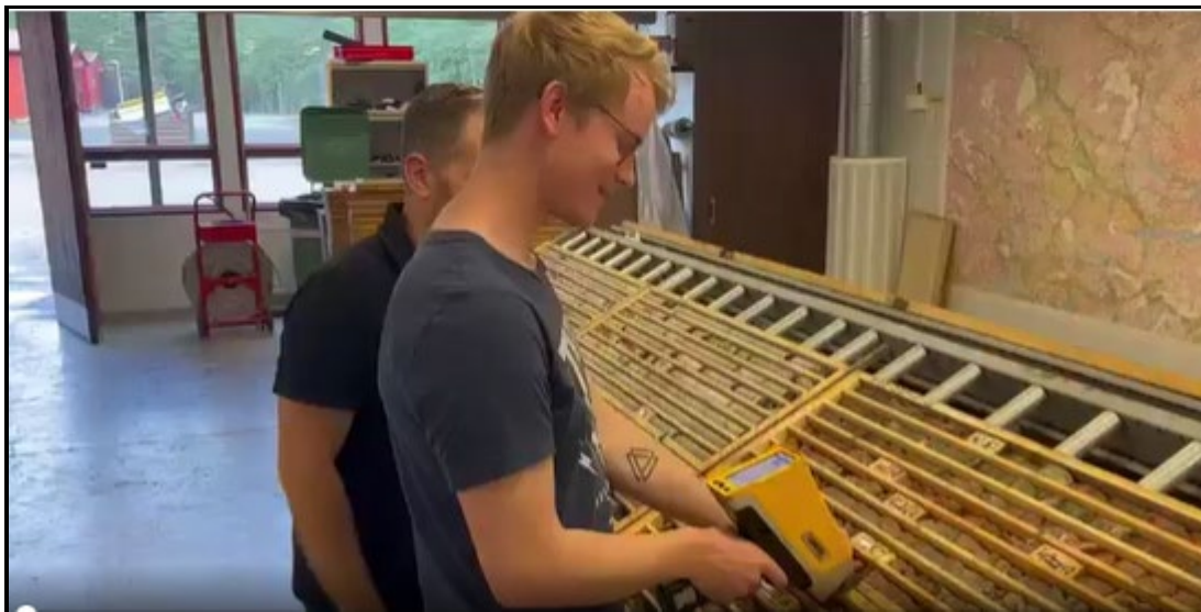
Niel van de Kerkhof of the Department of Earth and Environmental Sciences, KU Leuven, Belgium sampling drill core with a portable XRF.
