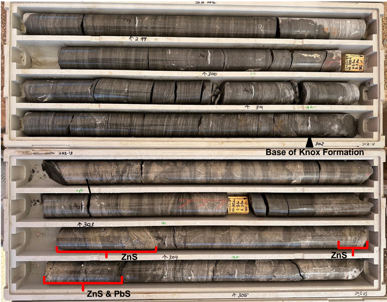
Figure 4 - Photograph of drill core interval 298.8 m to 305.35 m showing massive sphalerite + galena mineralisation intervals.
