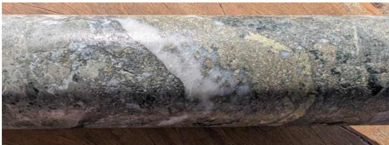
Figure 4 – Main lode in DTDD045 (94.6 - 94.9m), including brecciated quartz vein with associated pyrite and chalcopyrite in sericite altered andesite volcanics.
