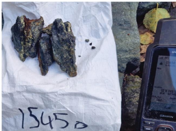
Sample 15450 from Tesskrokan (3.03% Cu)
