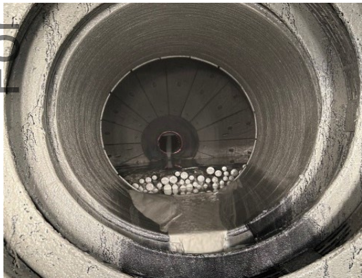
Picture 1: Rod mill charge level increase
