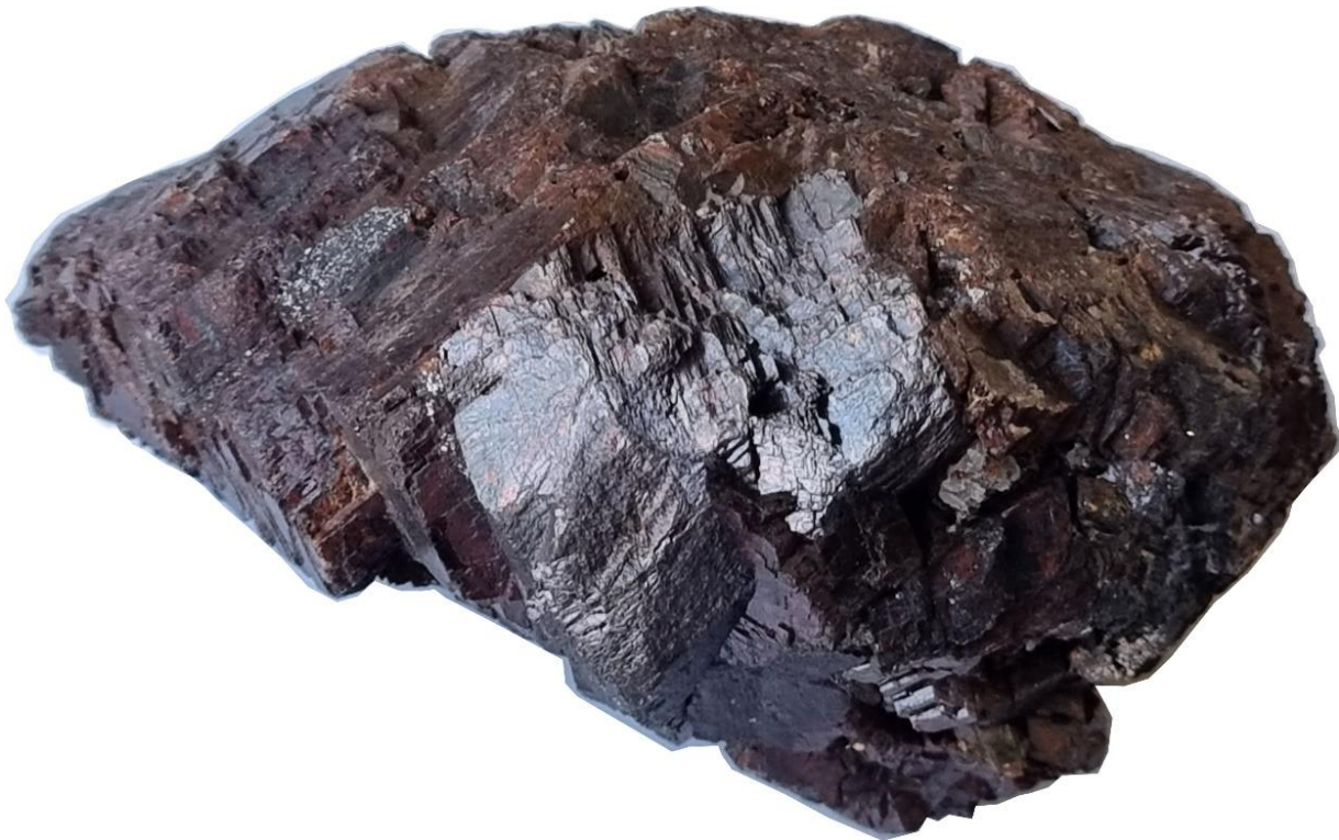
Figure 20: Mineralised waste dump specimen visually estimated to consist of 90% siderite and 10% cryolite.
