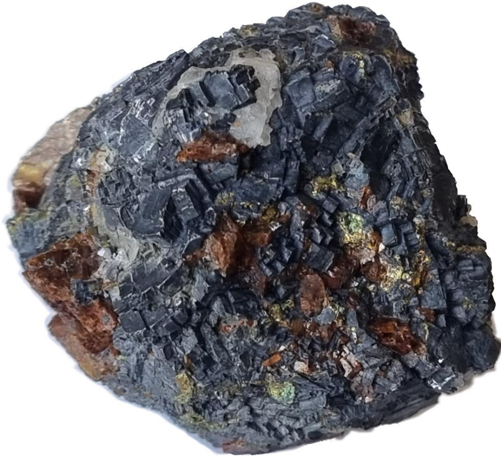
Figure 19: Mineralised waste dump specimen visually estimated to consist of 70% Galena; 10% Chalcopyrite; 10% Sphalerite and 10% Quartz.
