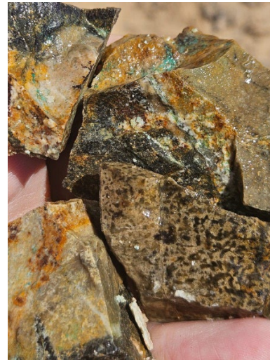
Figure 6: Hornfels, some with secondary biotite, with green and black copper oxides in fractures associated with quartz. Multiple generations of fine quartz veining indicate more than two hydrothermal events (262100E, 8060641N)
