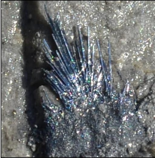
Figure 1: Stibnite (antimony sulphide) needles in fracture in core from BPD08. Antimony containing minerals at Bulla Park are tetrahedrite and stibnite
