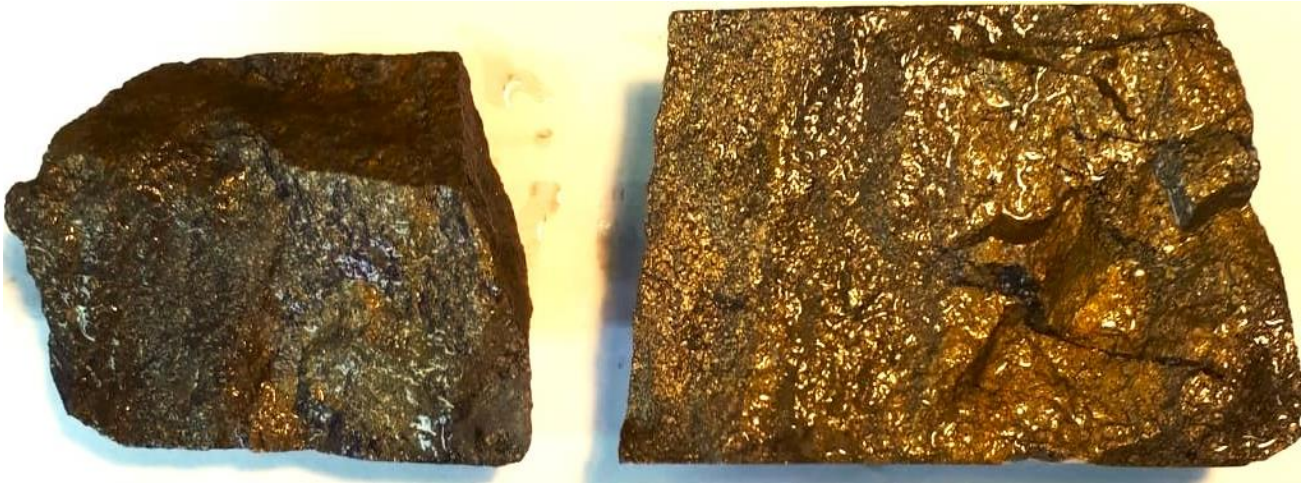
Figure 5: High grade drill core samples from hole ID97-20, 89.36 to 90.53 m (not the complete interval). This complete interval assayed 7.23% Cu, 1.17 g/t Au, 31.2 g/t Ag in the original assay information from Chemex Laboratories. The sulphide mineralisation is massive, concordant with the host unit and consists of chalcopyrite (25%), pyrite (5%). Re-sampling for re-assaying of the core was undertaken in September, with results expected in October. Hole located at 376995 East/6862748 North UTM Zone 9 and original project NAD27 datum.
