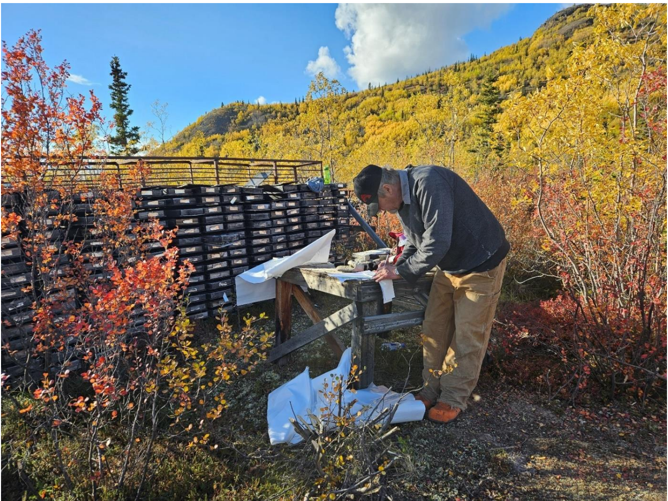
Figure 2: Core racks with labelled core trays and core resampling underway in the ICE property.
