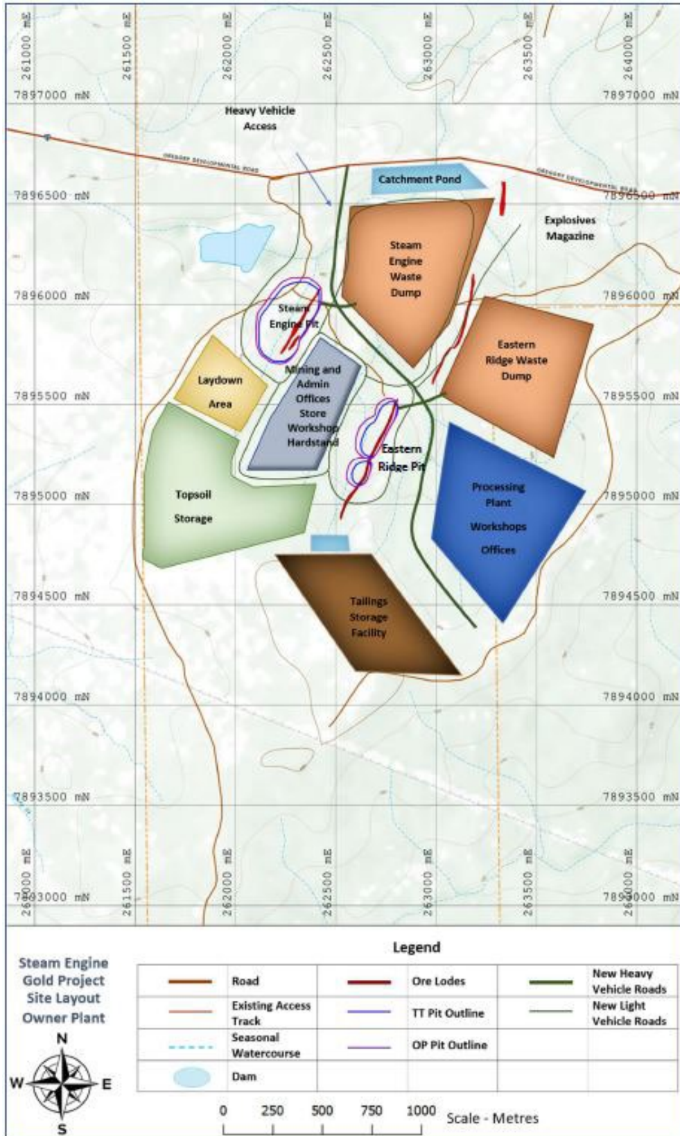
Figure 13. Steam Engine Gold Project conceptual site layout – Stand-Alone Processing scenario.
