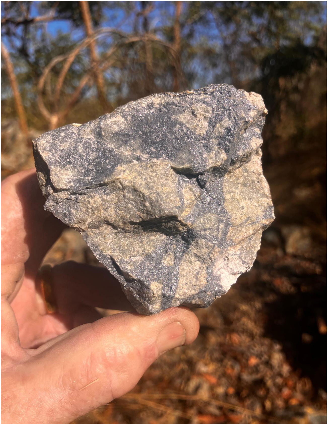
Chloritic altered rhyolite breccia with massive stibnite as matrix infill on southern lode (Vein System 2)
