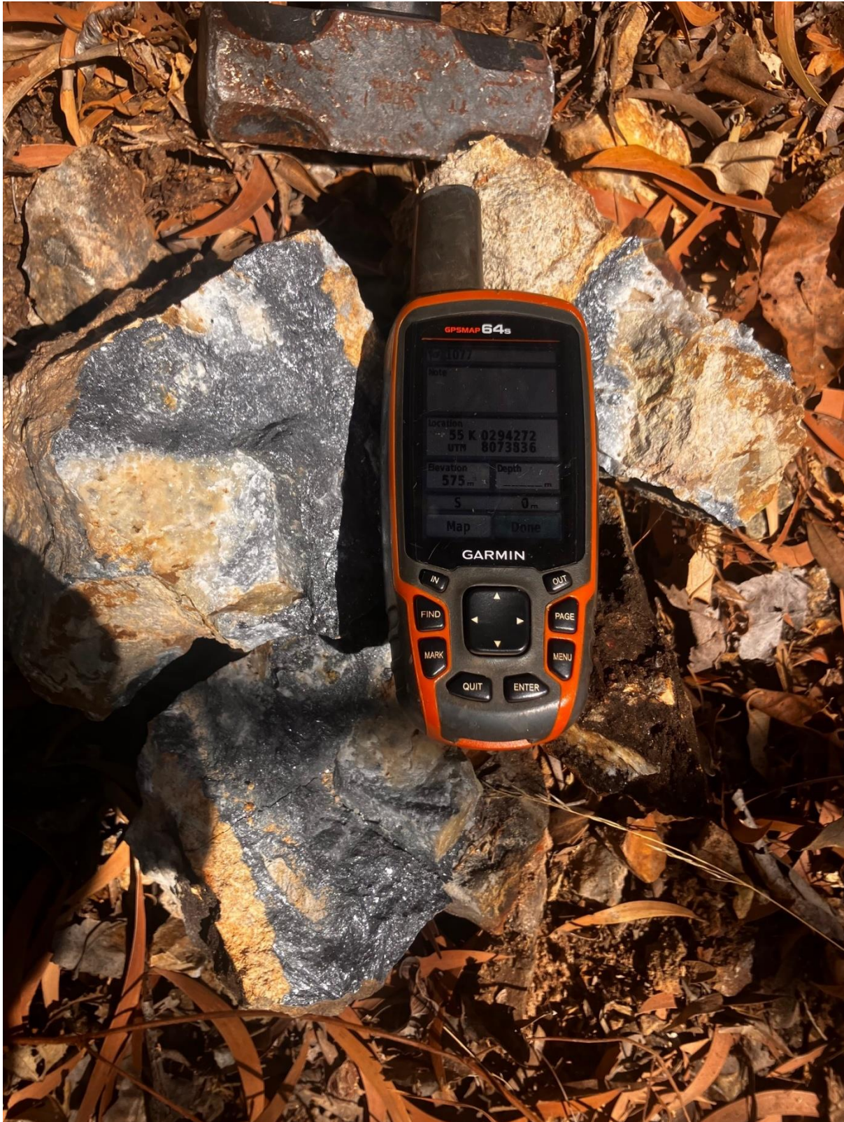
Brecciated quartz vein to 1m wide, massive to subhedral stibnite crystals grading to stibiconite on weathered surface. (Vein System 1)
