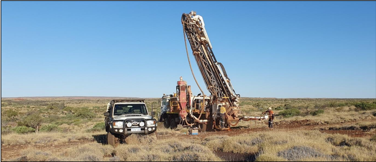
Figure 1: RC drill rig on tenement E46/1407 testing the W2 anomaly.
